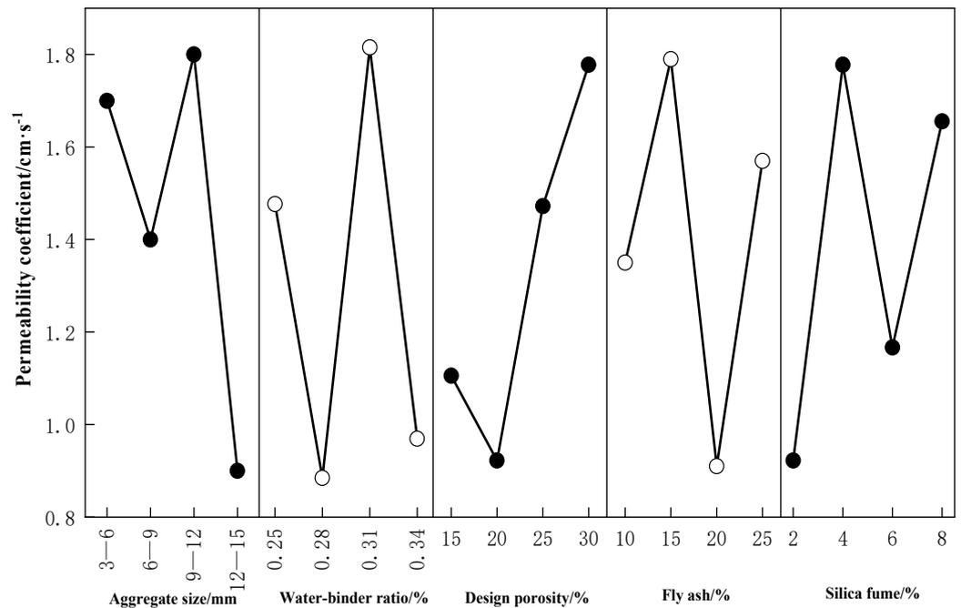
Figure 7. Influence of various factors on permeability coefficient of pervious concrete.
