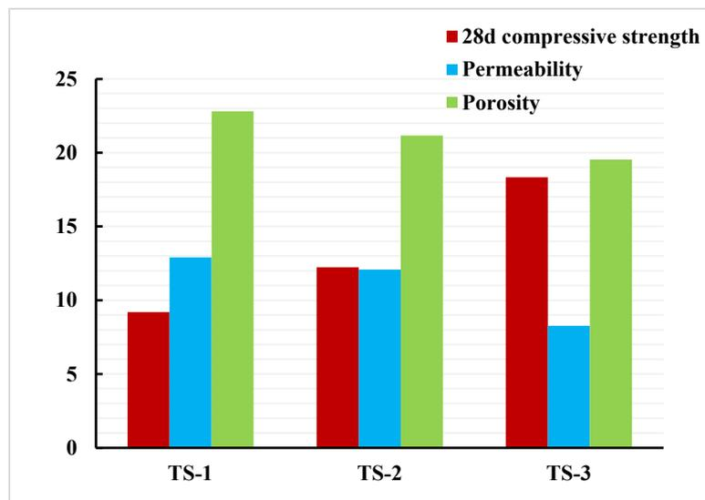
**Figure 9.** Histogram of performance test results of permeable concrete.
