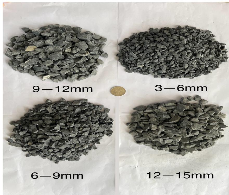
**Figure 1.** Different aggregate particle sizes.
