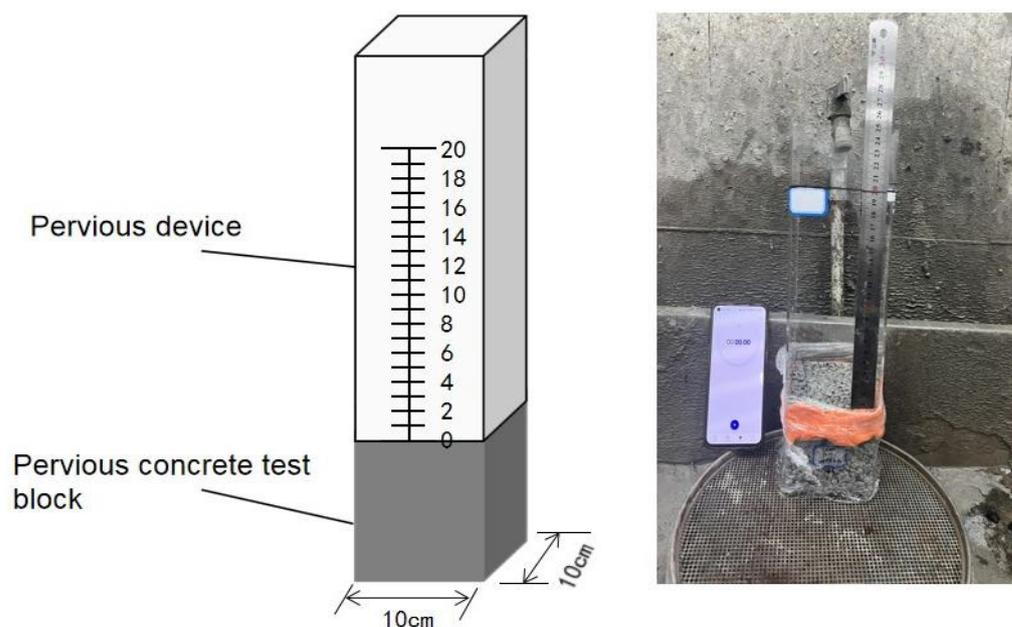
**Figure 5.** Self-made variable head osmotic flowmeter schematic and physical drawings.
