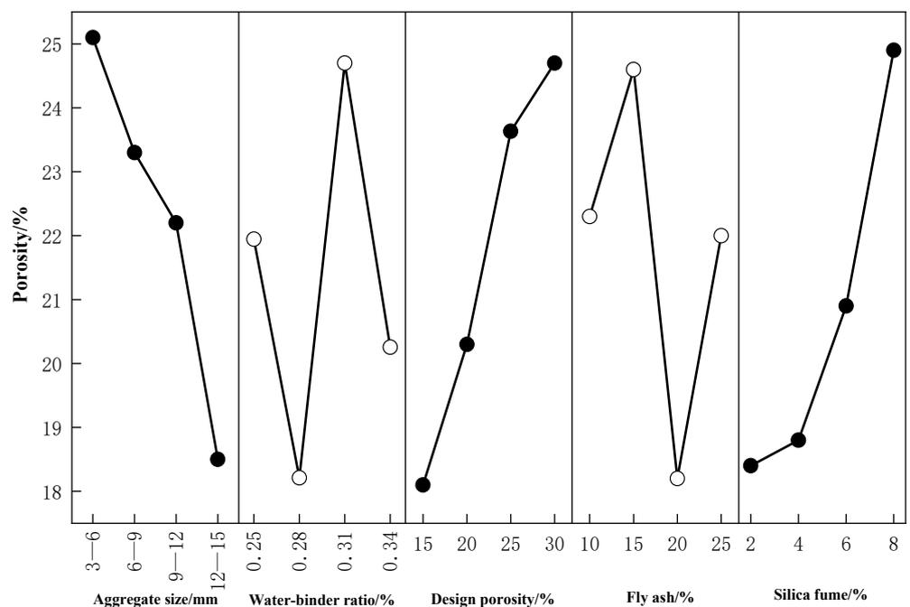
Figure 8. Influence of various factors on porosity of pervious concrete.
