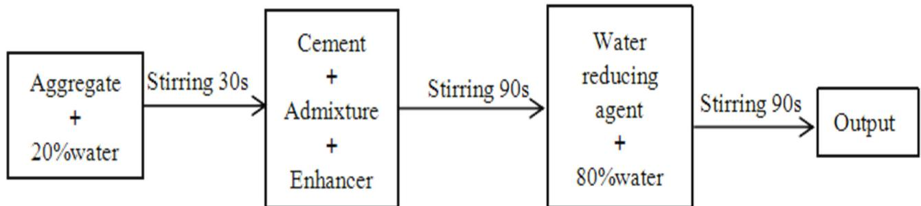
Figure 3. Cement-coated stone process flow diagram.
