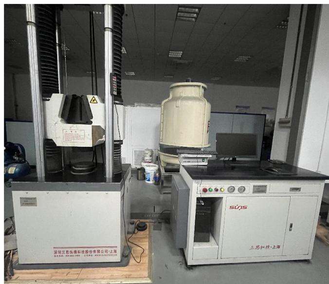
Figure 4. WAW-1000 electro-hydraulic servo universal testing machine.
