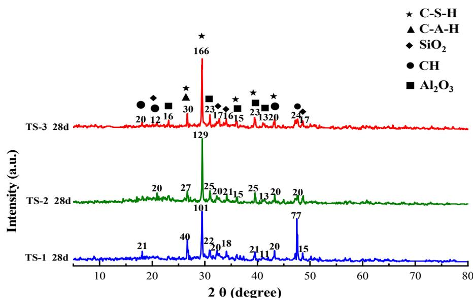
Figure 11. XRD pattern of hydration products of permeable concrete.
