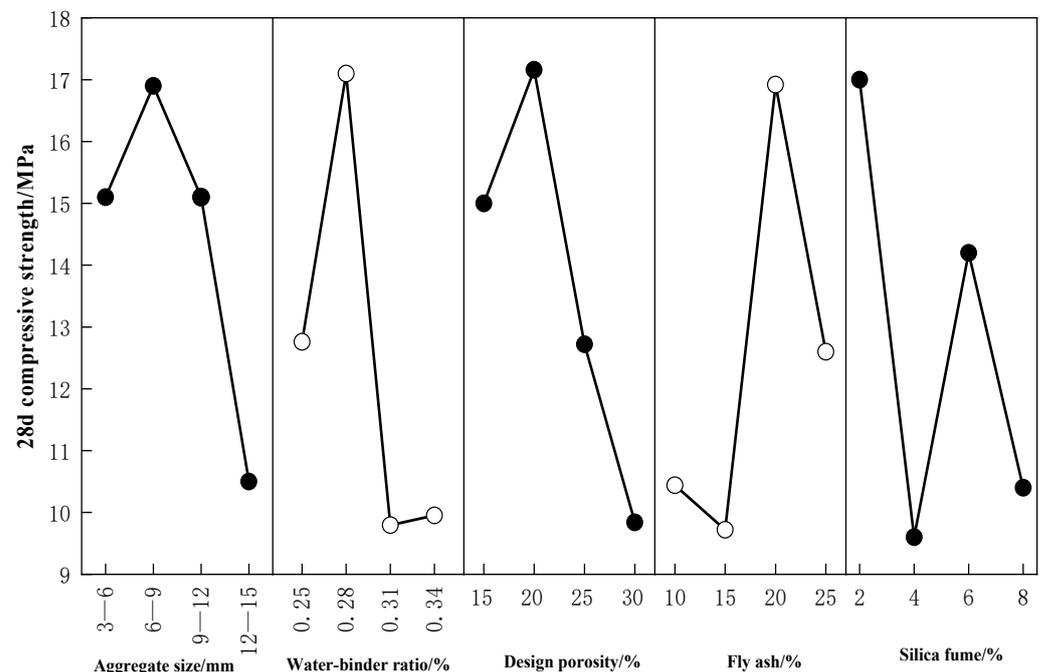
Figure 6. Influence of various factors on 28 d compressive strength of pervious concrete.
