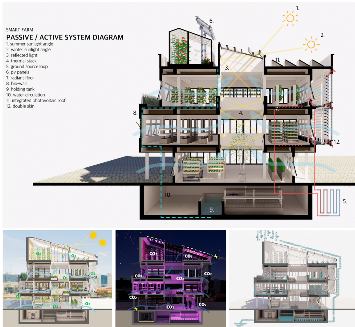
Figure 4. Image of rooftop greenhouse-type smart farm plan.
