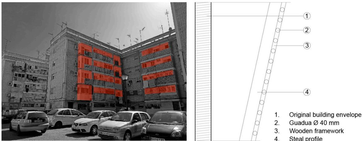
**Figure 8.** Some DIY renovations degrade the facades in the neighbourhood, and possible construction detail of the double skin.
