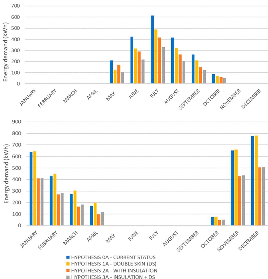
**Figure 14.** Monthly energy demand for cooling (kWh), (**up**), monthly energy demand for heating (kWh), (**down**).
