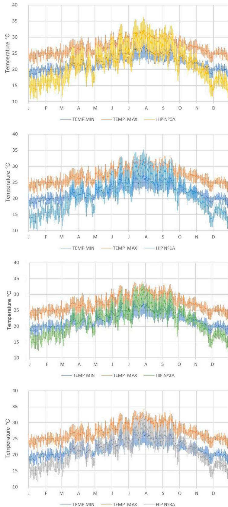
**Figure 13.** Thermal behaviour of the hypotheses studied in building B in relation to the minimum and maximum comfort temperatures.
