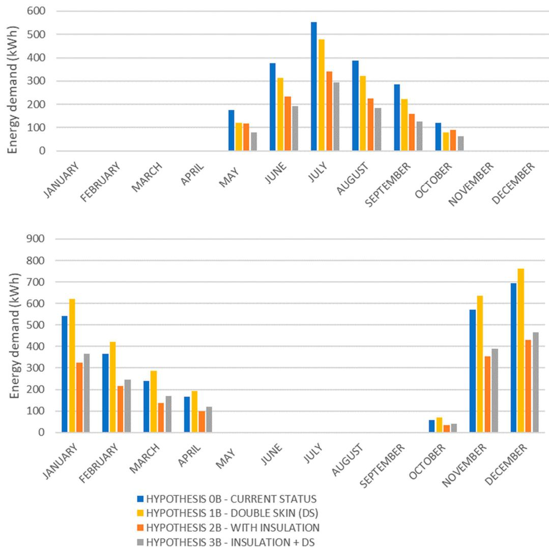
**Figure 15.** Monthly energy demand for cooling (kWh), (up), monthly energy demand for heating (kWh), (down).
