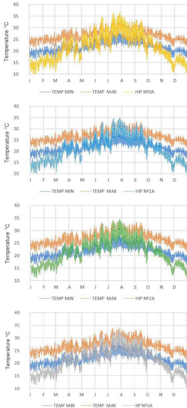
**Figure 12.** Thermal behaviour of the hypotheses studied in building A in relation to the minimum and maximum comfort temperatures.
