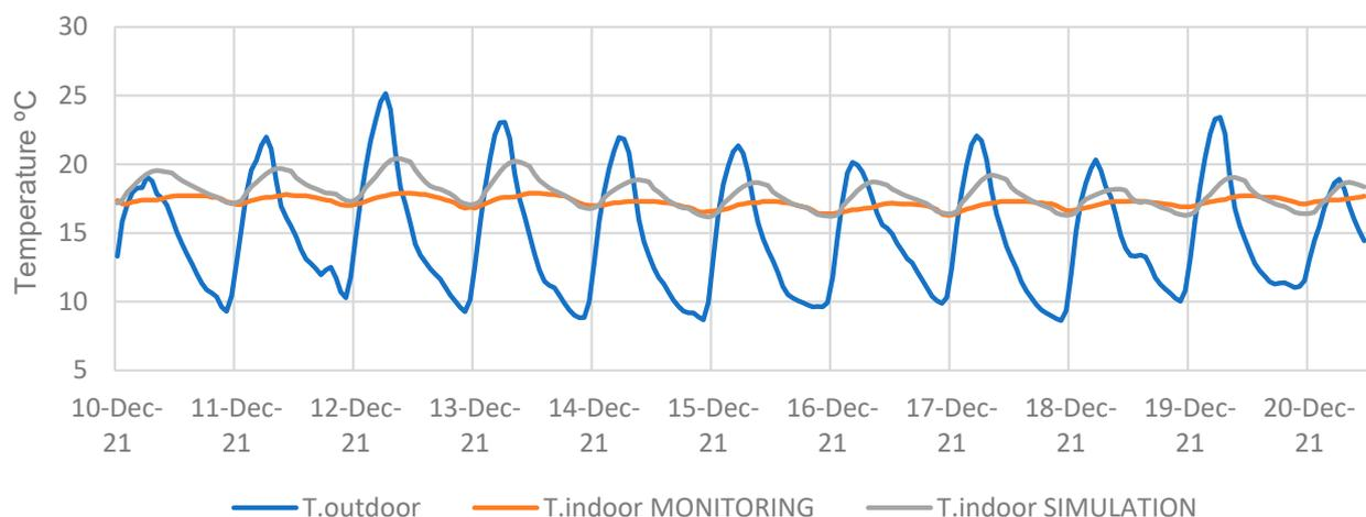
**Figure 10.** Temperature outdoor and temperature indoor in free evolution, in comparison to the simulation model temperature indoor.
