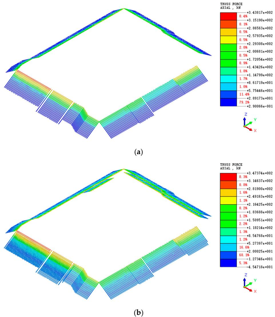
Figure 9. Nephogram of maximum axial force of anchor bolt: (a) First layer; (b) Second layer.
