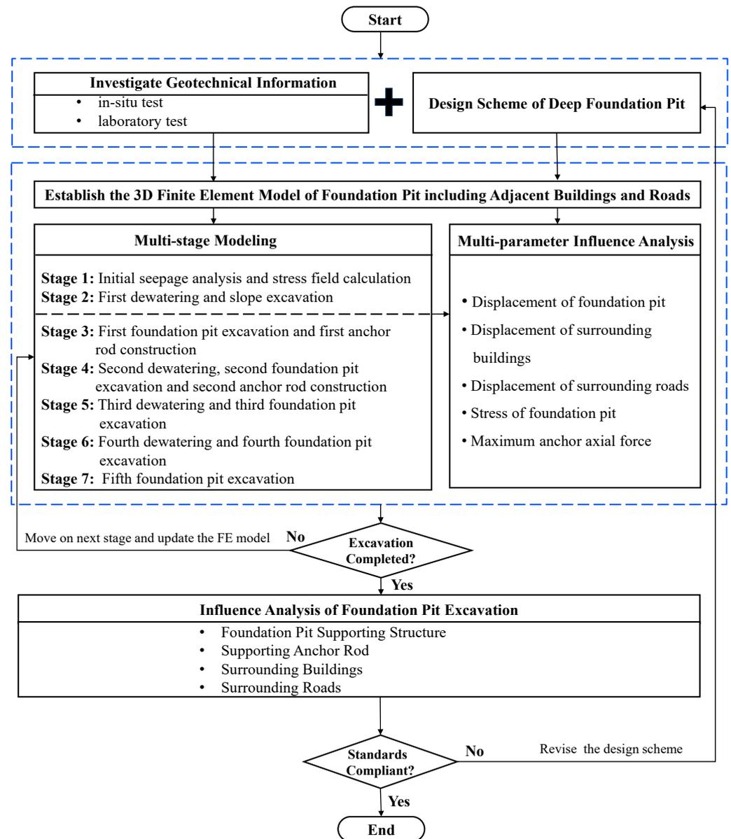
**Figure 2.** Flowchart of the proposed multi-stage and multi-parameter influence analysis of deep foundation pit excavation.
