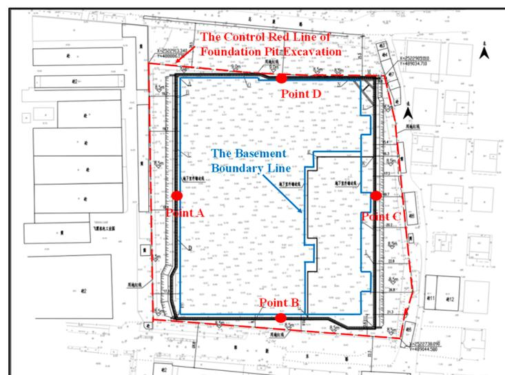
**Figure 6.** Feature points of numerical simulation.
