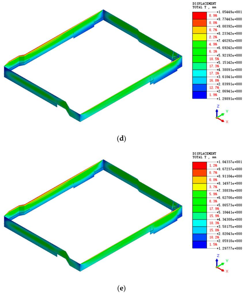
**Figure 5.** Displacement nephogram of maximum total displacement values for foundation pit support at each stage for pit support structures: (a) Stage 3; (b) Stage 4; (c) Stage 5; (d) Stage 6; (e) Stage 7.
