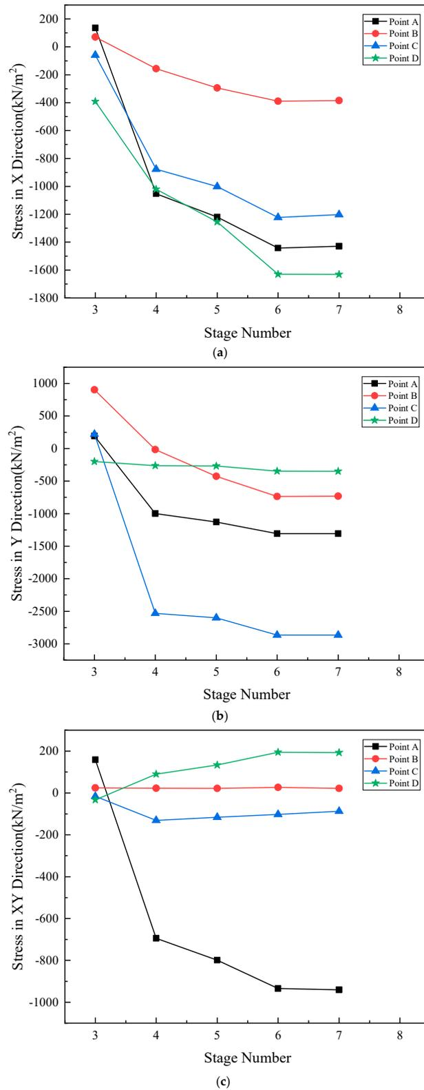
**Figure 8.** Pit support stress cartogram: (a) X-direction; (b) Y-direction; (c) XY-direction.
