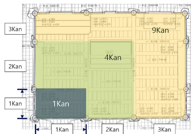
Figure 12. A 3 × 3 (9-kan) floor plan [16]. In the elevation of a hanok, a unit of 1 kan is used between columns. Additionally, 1 kan also means a unit of space. Therefore, this floor plan is 3 kan in the front and 3 kan on the side, or 9 kan in size.
