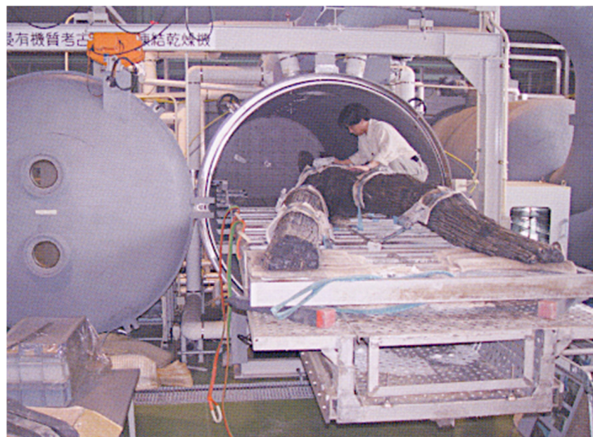
Figure 21. Testing authentic wooden relics from the Nara Palace site (source: Nabunken, 2004).
