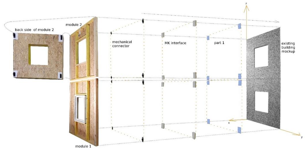
Figure 8. Exploded view of the 2D module in Test 3.
