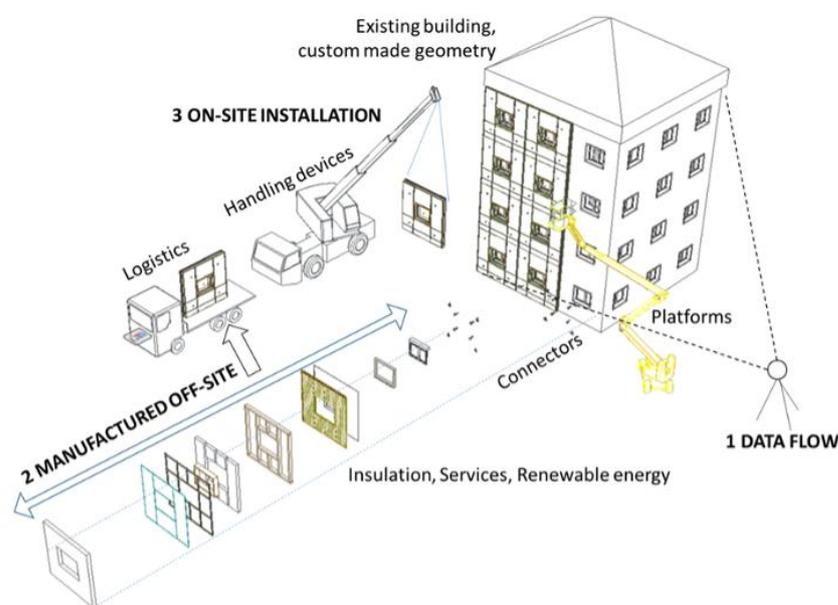
**Figure 1.** Building renovation process with prefabricated panels for the envelope.
