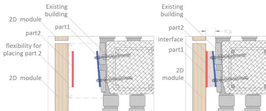
**Figure 5.** Left: Flexibility for placing Part 2. Right: The shape of the interfaces.
