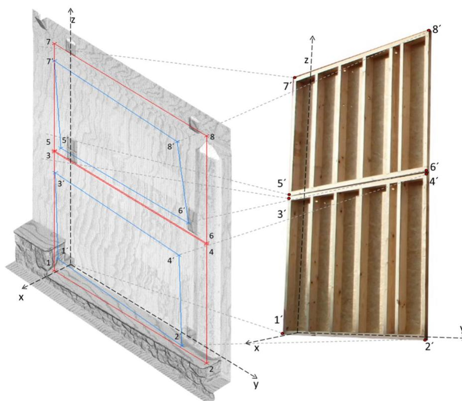
**Figure 21.** On the left: graph of the planned layout in red and placed deviation in blue magnified by a factor of 20 in Test 4. On the right: picture of the installed prefabricated modules with the corresponding points.
