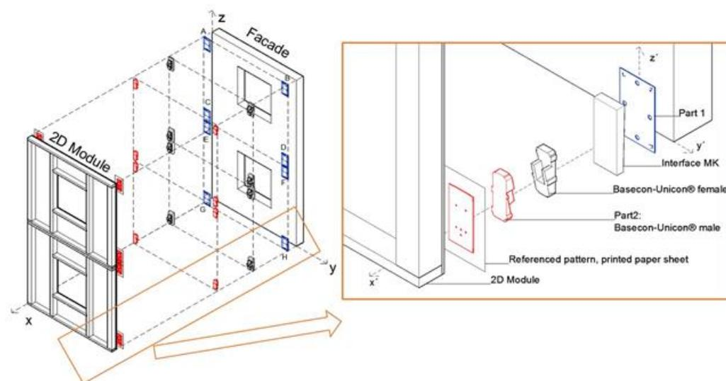
Figure 7. Exploded view of the 2D module in Test 3.
