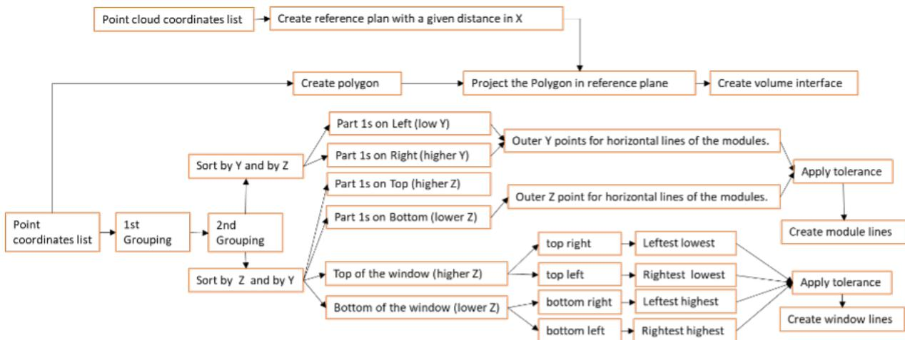
Figure 13. Process flowchart.
