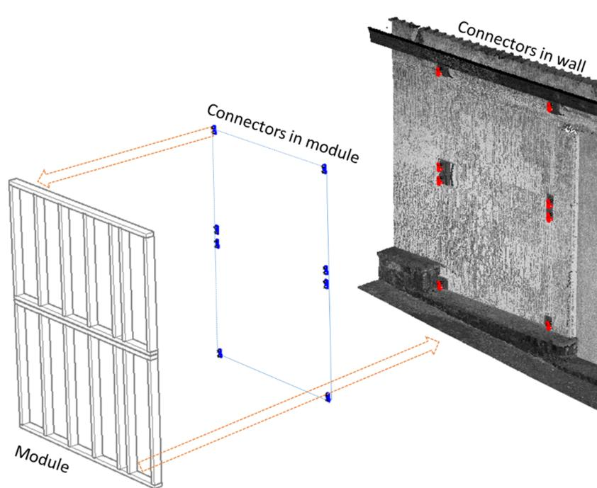
**Figure 2.** Exploded view of a module being placed in a wall with connectors. Point Cloud made in BERTIM project [22].
