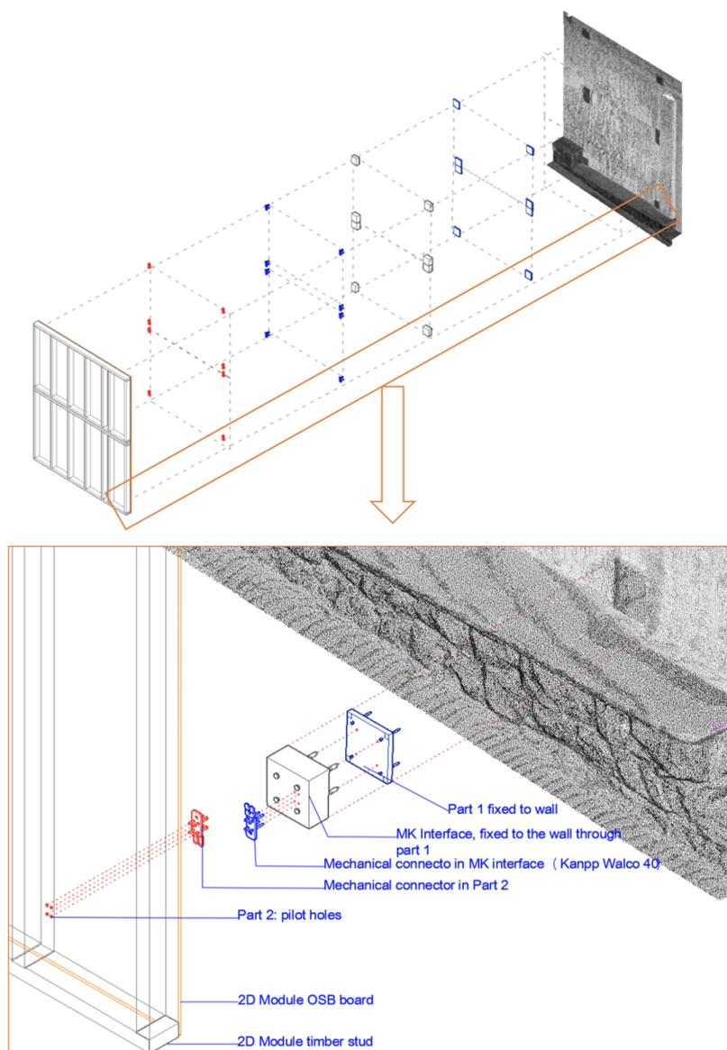
**Figure 15.** Installation process of the Matching Kit at Test 4.
