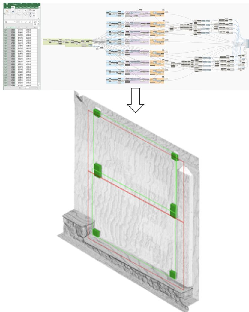
**Figure 17.** The figure shows the output of the automated process of layout generation, from the Excel file to the layout and MK definition. In red: the perimeter of the prefabricated modules. In green: the MK interfaces and accessory lines.
