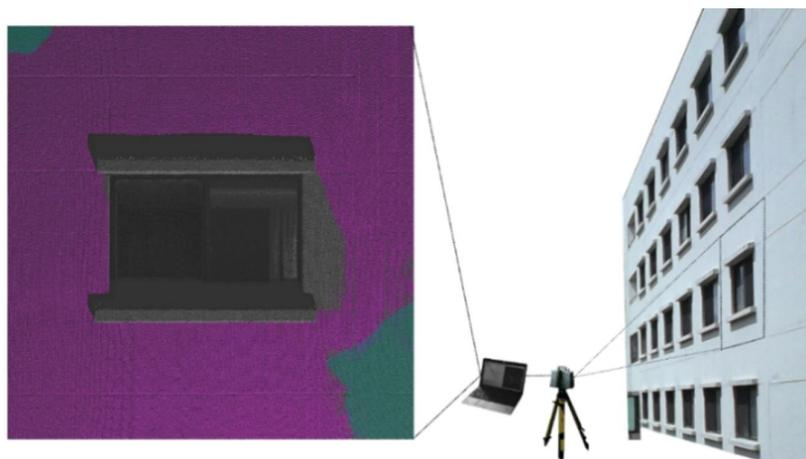
**Figure 3.** Data from a 3D laser scanner showing non-planar situation of a segment of a wall, with the help of Prof. Kwon at SKKU.
