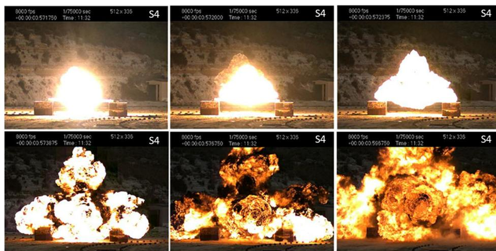
**Figure 7.** Image sequence of the high-speed camera during test S4 (15 kg eq. TNT at 1 m).
