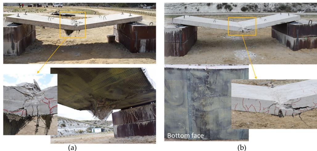
**Figure 15.** Post-blast images of slabs protected with CFRP with the charge at a standoff distance of 1 m: (a) test P6; (b) test P8.
