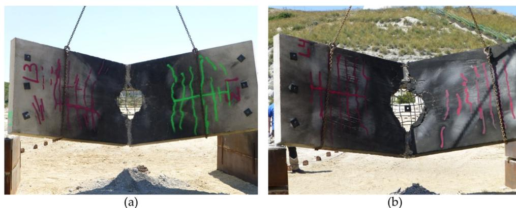
**Figure 13.** Post-blast images of slabs protected with fiber-reinforced concrete: (a) S7 with steel fibers; (b) S8 with polypropylene fibers.
