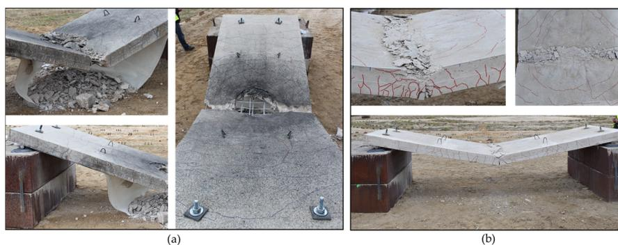
**Figure 14.** Post-blast images of slabs protected with GFRP: (a) result with the charge at a standoff distance of 0.5 m; (b) result with the charge at a standoff distance of 1 m.
