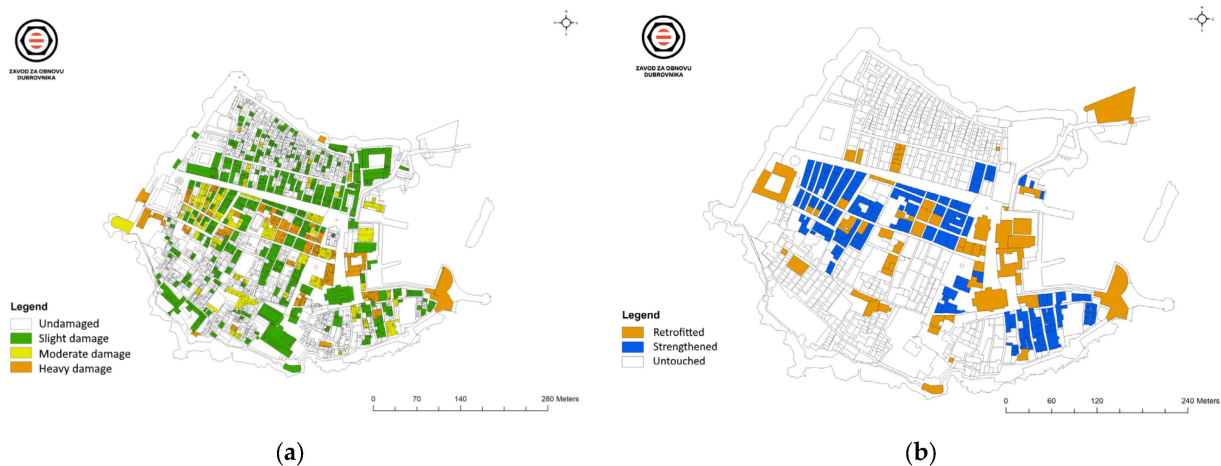
Figure 10. The Old City of Dubrovnik following the 1979 M7 Montenegro earthquake: (a) state of damage to buildings; (b) seismic intervention to buildings available at [46].
