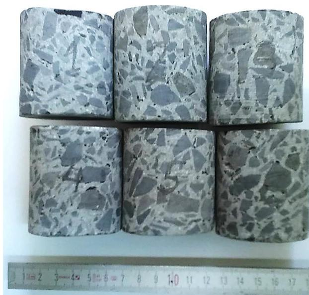
**Figure 2.** View of samples taken from the floor slabs.
