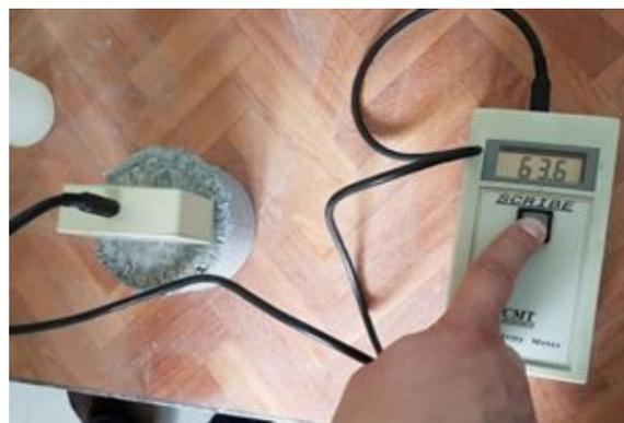
**Figure 6.** Value of read resistance of concrete expressed in  $k\Omega\text{cm}$ .
