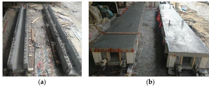
**Figure 2.** Fabrication of the specimen. (a) UHPC channel beam; (b) RCCD slab.
