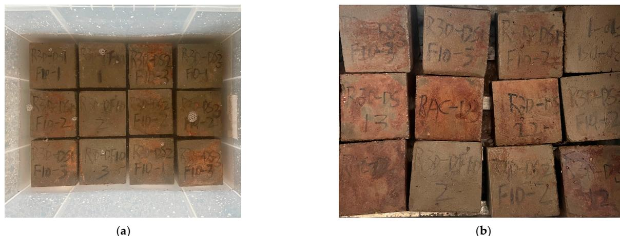
**Figure 3.** Freeze–thaw testing. (a) Specimen immersion; (b) specimen freeze–thaw.
