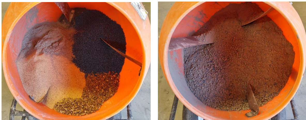
Figure 3. Dry mixing of concrete ingredients with crumb rubber.
