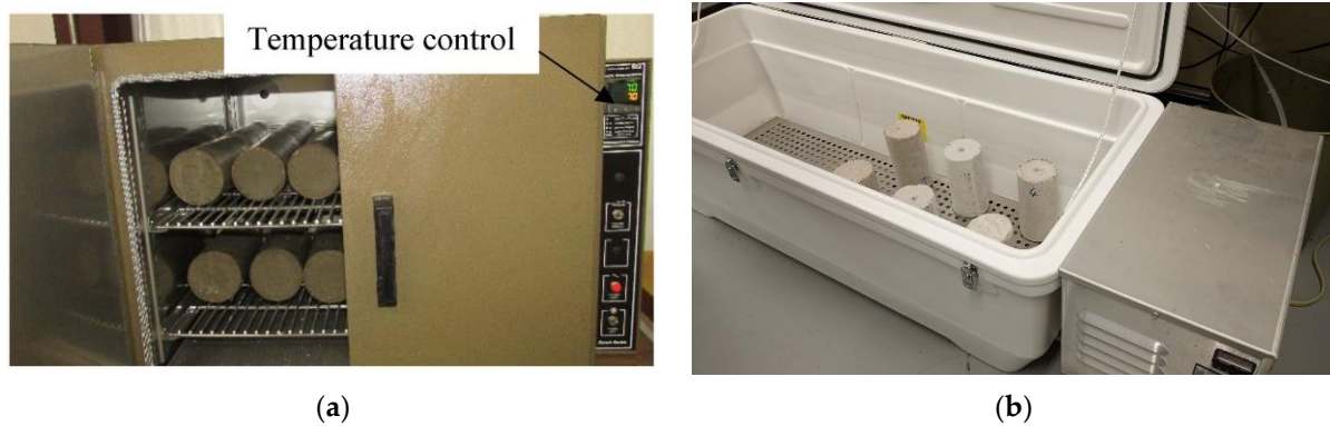
Figure 4. Temperature control equipment. (a) Temperature control ovens. (b) Freeze–thaw testing machine.
