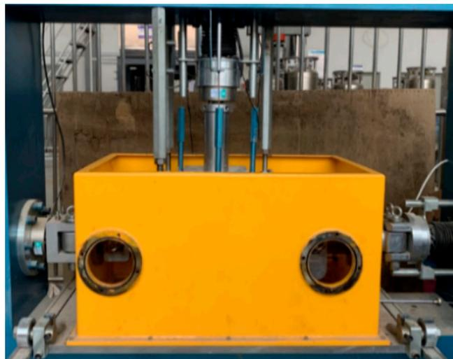
**Figure 2.** XHZJ-30 large circular shear tester.
