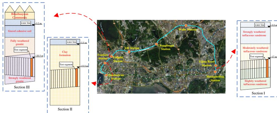
**Figure 1.** Route map and three sections of Shenzhen Metro Line 5.
