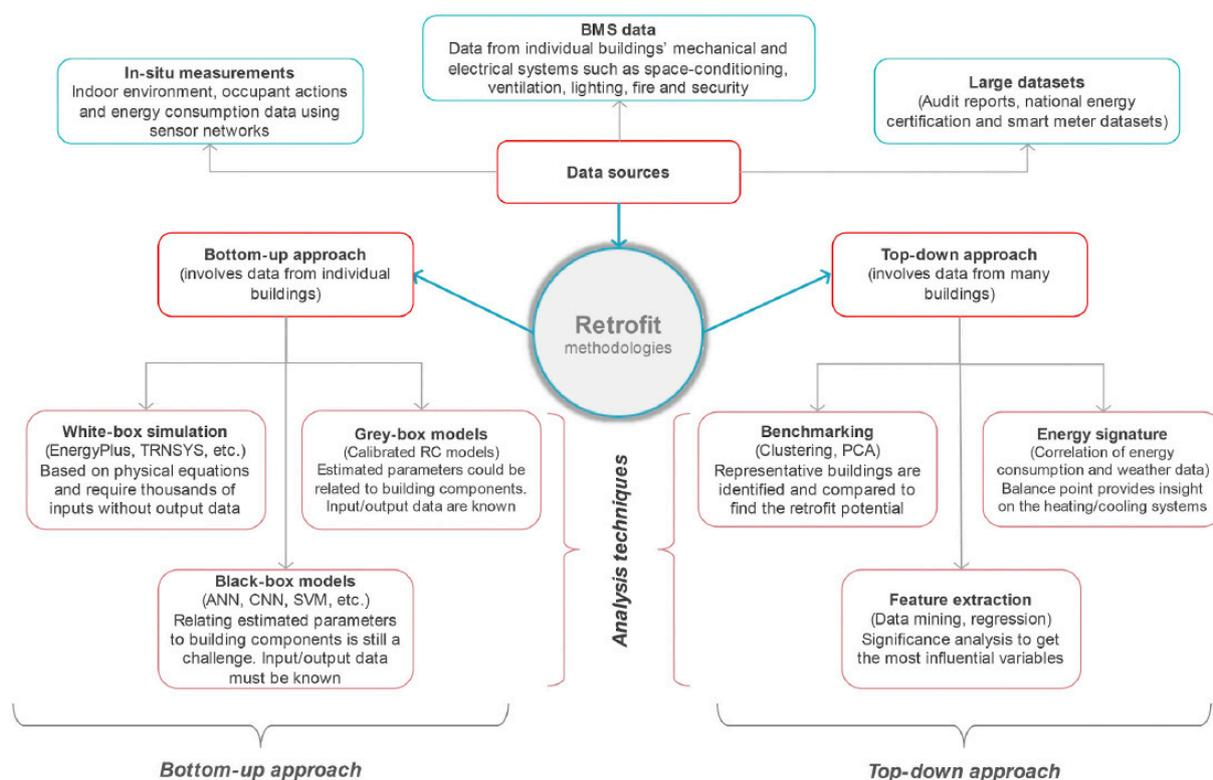
Figure 10. Illustration of different retrofit approaches [87].
