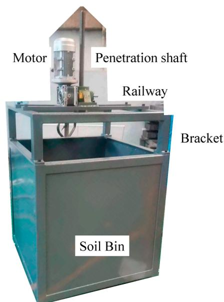
Figure 1. Experimental apparatus.
