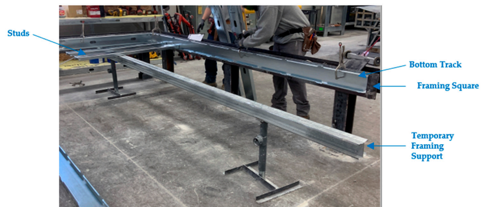
Figure 7. Wall panel assembly in plant.
