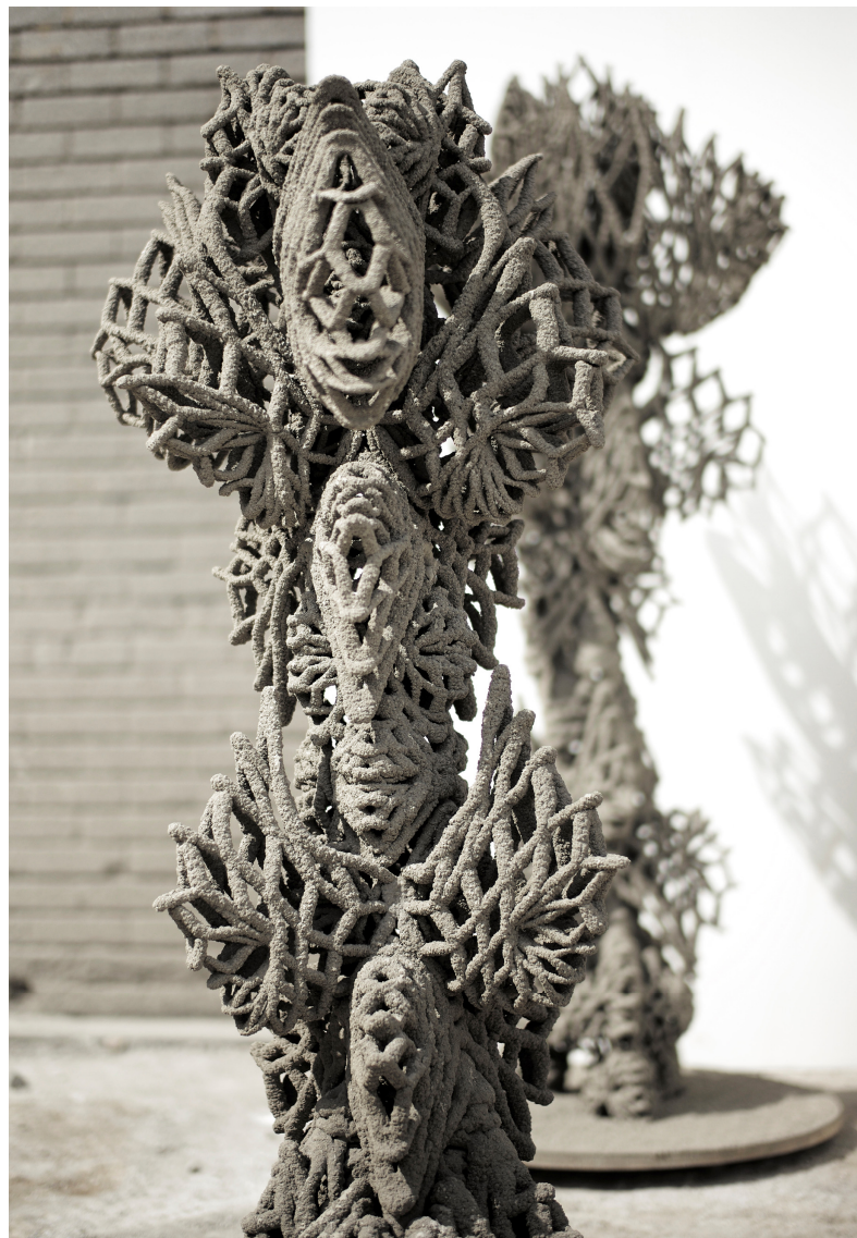
Figure 18. Two columns sprayed with different mixtures: the front one is sprayed with PVA and the back is not.
