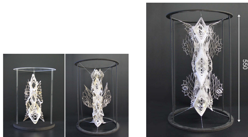
Figure 10. Different columns/units which are made of one piece of paper (for the simulation). There are multiple hexagons on one paper. The lines are drawn on the paper via laser cutting.
