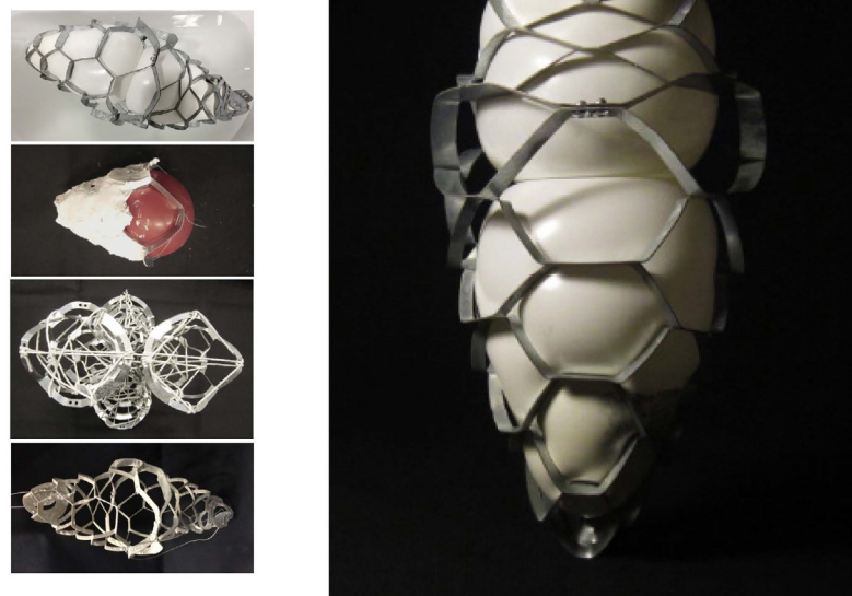
Figure 16. A possible method of casting: putting the balloon into the steel structure and then pouring the cement mixture into it.
