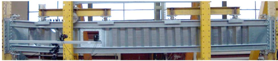
**Figure 6.** Deformed shape of the CWB-SW-WO assembled by spot welding.
