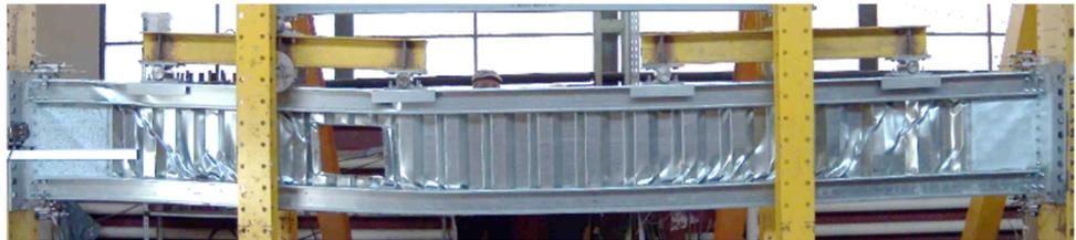
**Figure 7.** Deformed shape of the CWB-CMT-WO assembled by MIG brazing.
