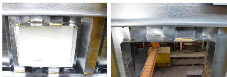
**Figure 5.** Reinforcement the web opening for the CWB-CMT-WO specimen assembled by MIG brazing.
