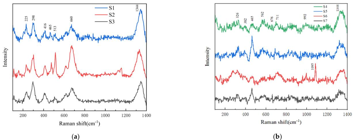
**Figure 7.** Raman spectra of clinker bricks. (a) S1–S3; (b) S4–S7.
