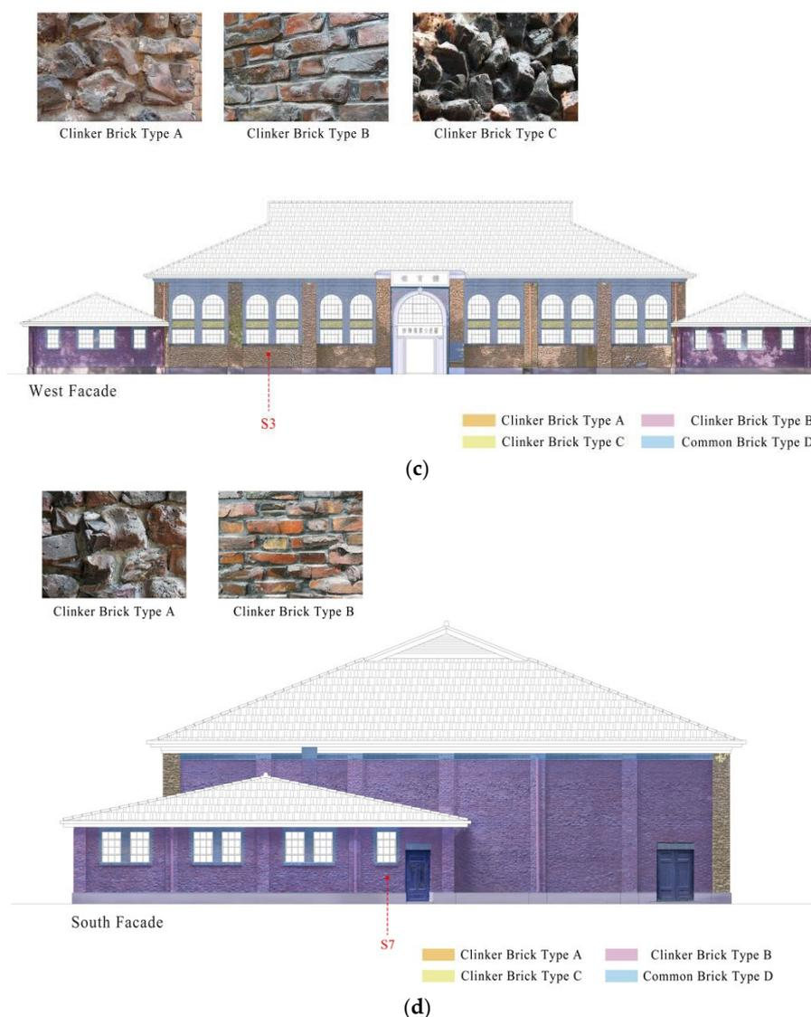
**Figure 4.** Morphological types of bricks and localization of the samples on the facades of the Smart Memorial Gymnasium. (a) North facade; (b) East facade; (c) West facade (main facade); (d) South facade.
