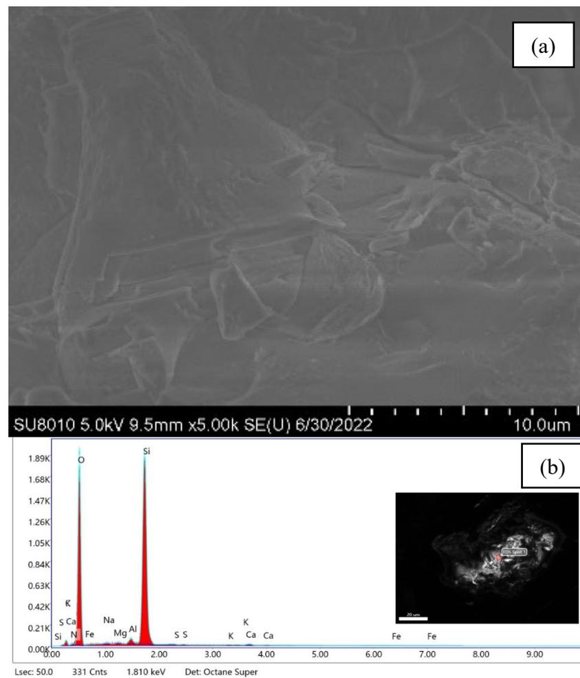
**Figure 5.** (a) SEM of the clinker brick (sample S1); (b) EDS of the clinker brick (sample S1); the inset image is the collecting point.
