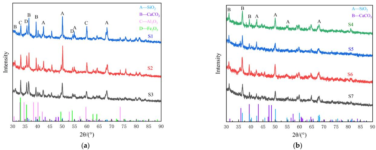
**Figure 6.** Measured XRD patterns of the clinker bricks (traces labelled S1–S7): (a) S1–S3; (b) S4–S7. The standard XRD patterns for the identified compounds are also shown at the bottom of the plots.
