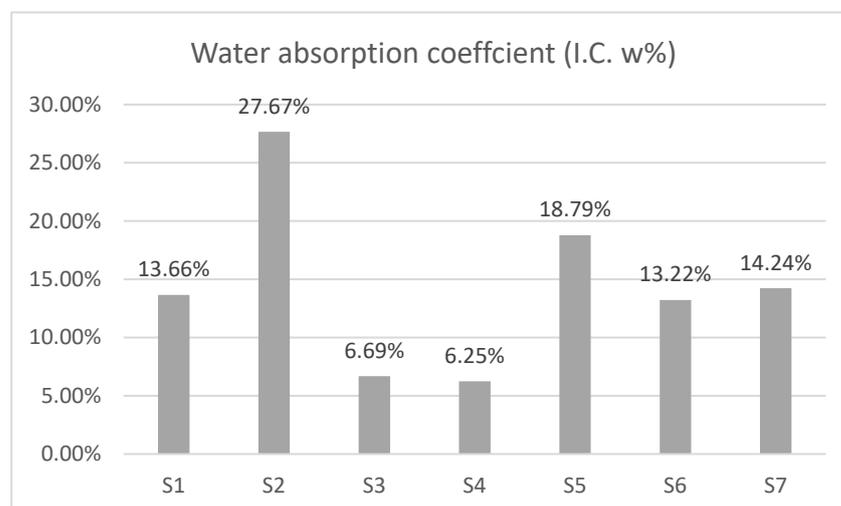
**Figure 8.** Water absorption coefficient of 7 samples.
