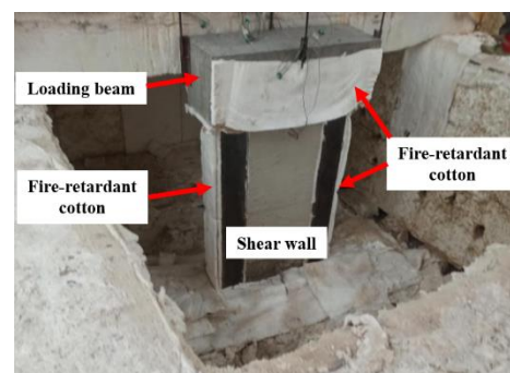
Figure 4. Fire protection treatment of specimen.
