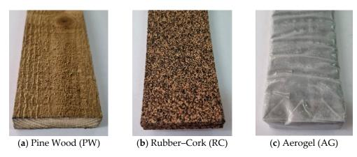
Figure 2. Thermal break strip materials assembled on the LSF partitions.
