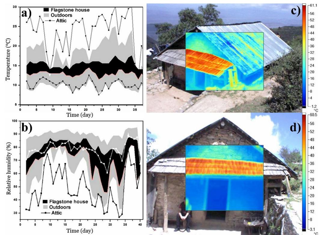
**Figure 5.** (a) Temperature and (b) relative humidity of the flagstone construction and outdoor environment. Lines show the values of the attic, locally named “*tapanco*”. Thermographic images of the flagstone construction in the *Sierra Gorda* of Querétaro, México. (c) Frontal view and (d) “*tejamanil*” shed over the door.
