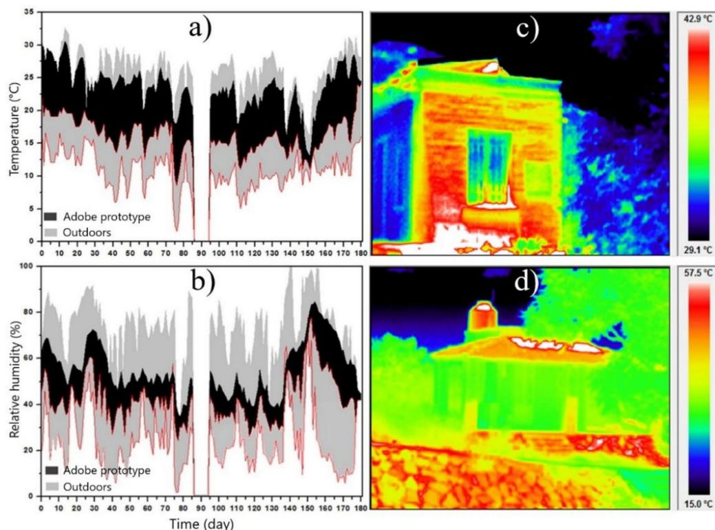
**Figure 3.** (a) Temperature and (b) relative humidity of the adobe prototype and outdoor environment. Thermographic images of the adobe prototype showing (c) the right side of the building, and (d) the facade of the building.
