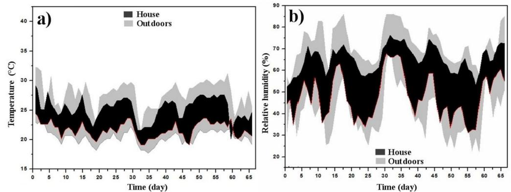
**Figure 7.** Bimonthly graphs of the behavior of the conventional house for (a) temperatures and (b) relative humidities.
