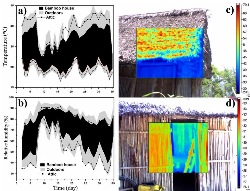
**Figure 6.** (a) Temperature and (b) relative humidity of the Bamboo (*Bambusa oldhamii*) house and outdoor environment. Lines are showing the values of the attic, locally named “*tapanco*”. Thermographic images of the bamboo house in the *Sierra Gorda* of Querétaro, México. (c) Roof view and (d) façade view.
