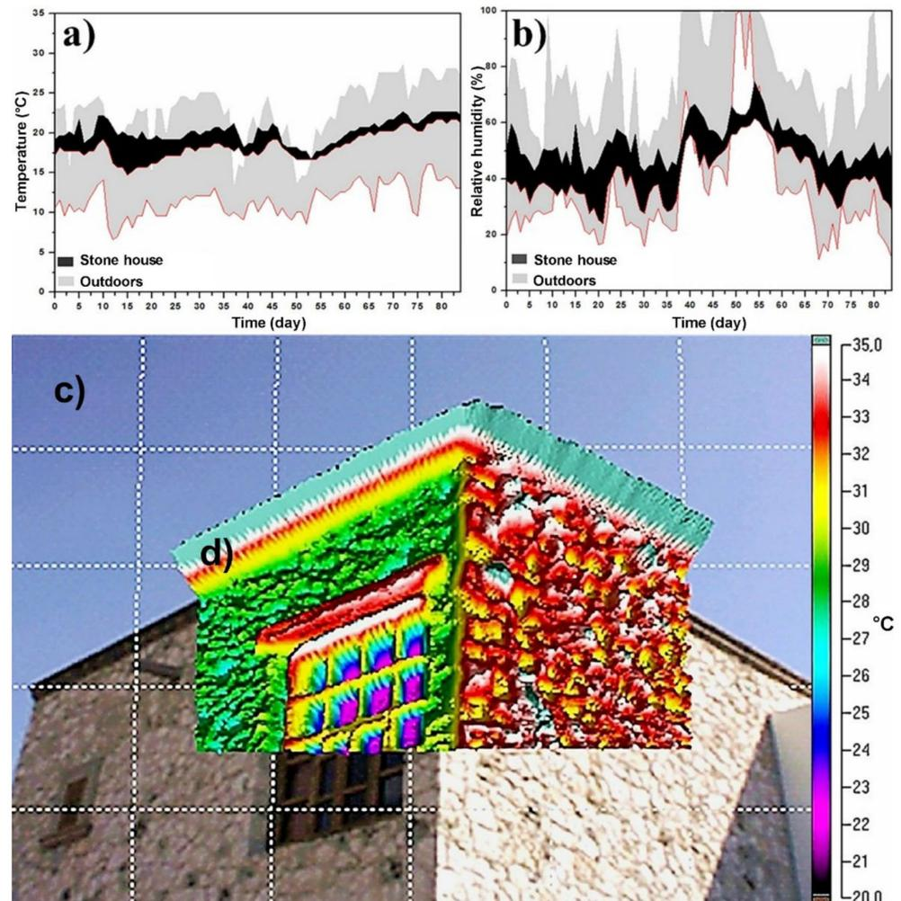
**Figure 4.** Quarterly graphs of the behavior of the stone house for (a) temperatures and (b) relative humidities. (c) Porous stone house, two-floor and (d) inserted thermographic image of the stone house.
