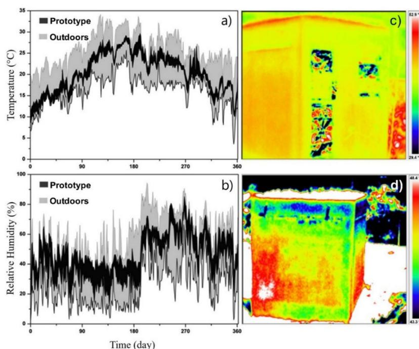
**Figure 2.** (a) Temperature and (b) relative humidity of the waste PET bottles prototype and outdoor environment. Thermographic images of the PET prototype showing (c) the right side and façade of the room and (d) the backside of the building.
