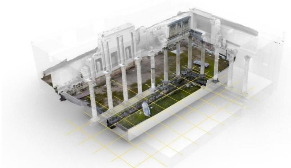
**Figure 9.** The photogrammetric survey carried out with UAV technology of the Mérida Forum Portico.
