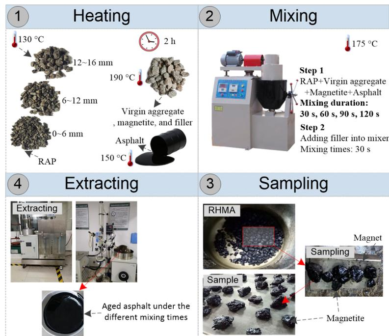
**Figure 4.** The process of blending asphalt with different mixing durations.
