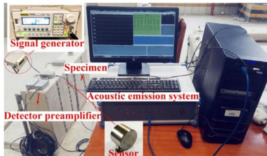
**Figure 3.** Acoustic emission system [62].
