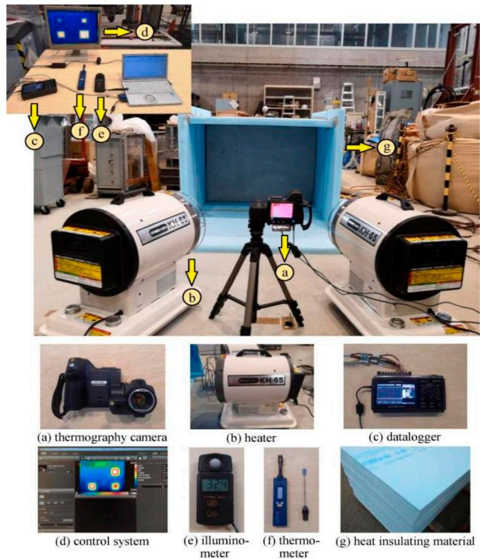
Figure 13. Setup of the experiment [121].
