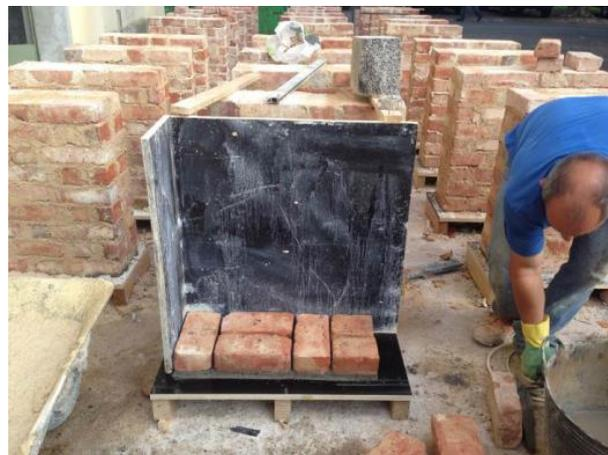
Figure 5. Execution of new solid brick wallettes.
