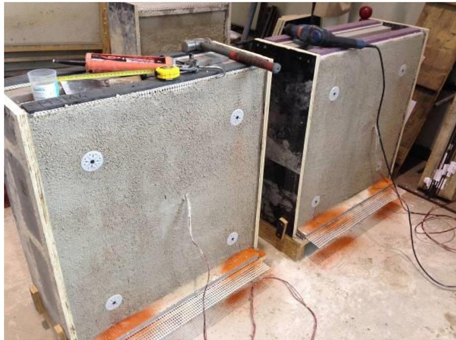
**Figure 6.** Wallettes with the reinforced render.
