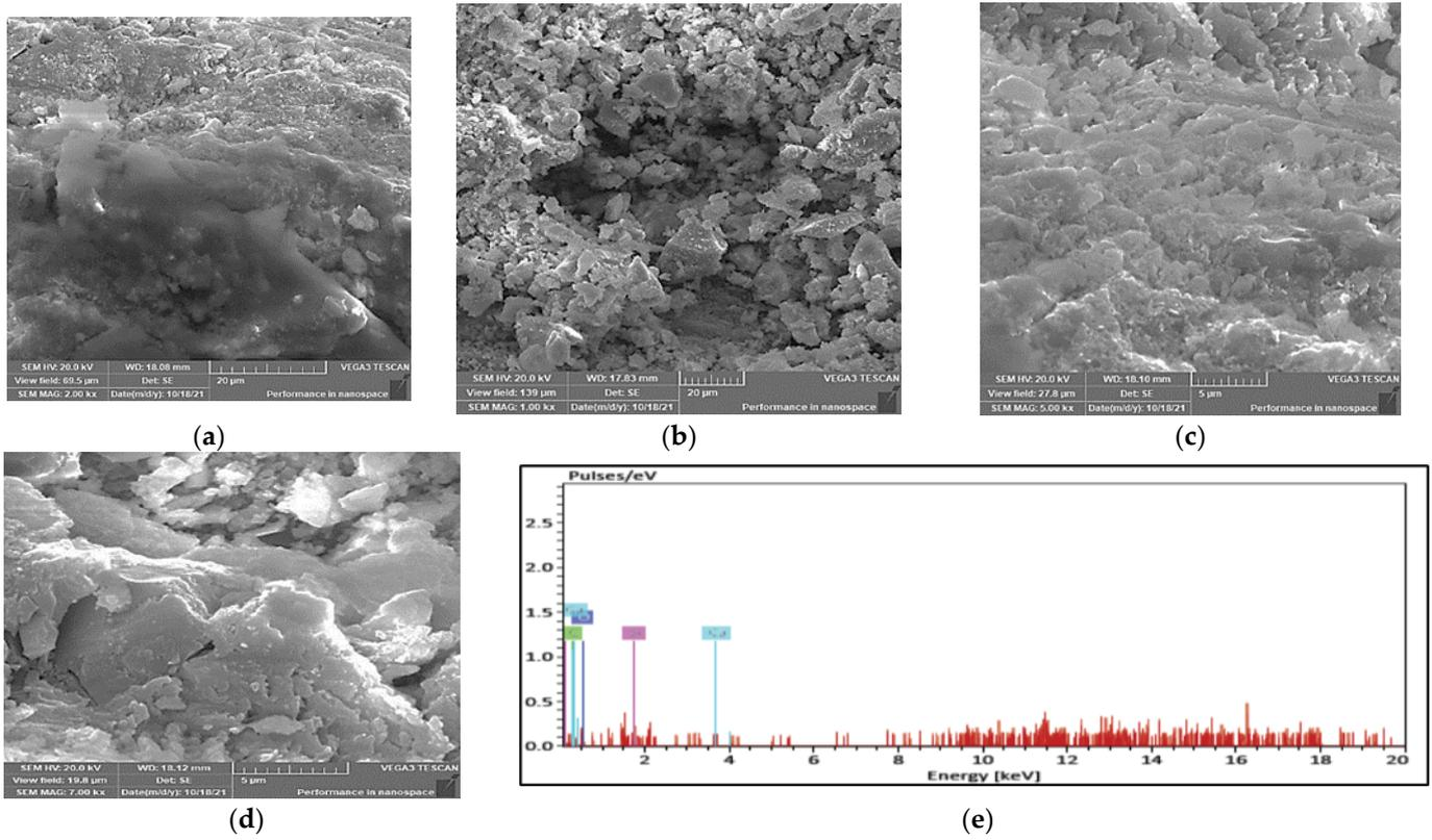
Figure 15. SEM with various magnification factors (a–d); (e) EDX for the mix UHPSCC 7 at normal curing temperature.
