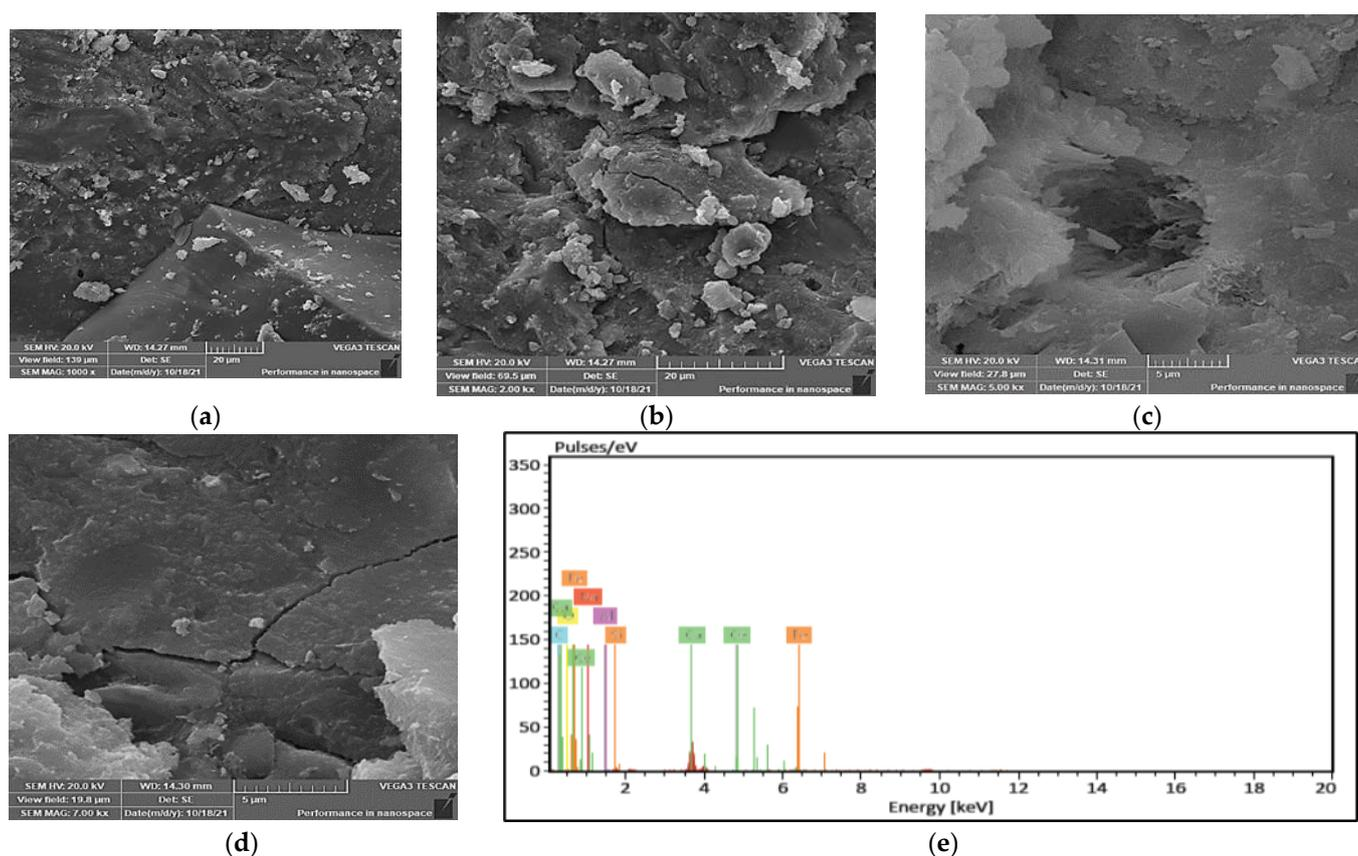
**Figure 17.** SEM with various magnification factors (a–d); (e) EDX for the mix UHPSCC 7 at (200 °C) temperature.
