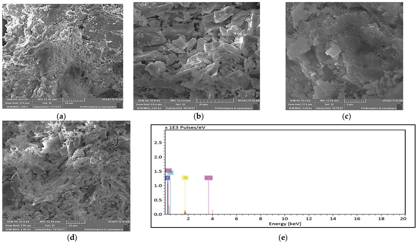
Figure 14. SEM with various magnification factors (a–d); (e) EDX for the mix UHPC 3 at normal curing temperatures.
