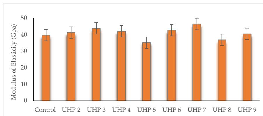
**Figure 7.** Modulus of elasticity after 90 days for glass and lime powder replacement ratios.
