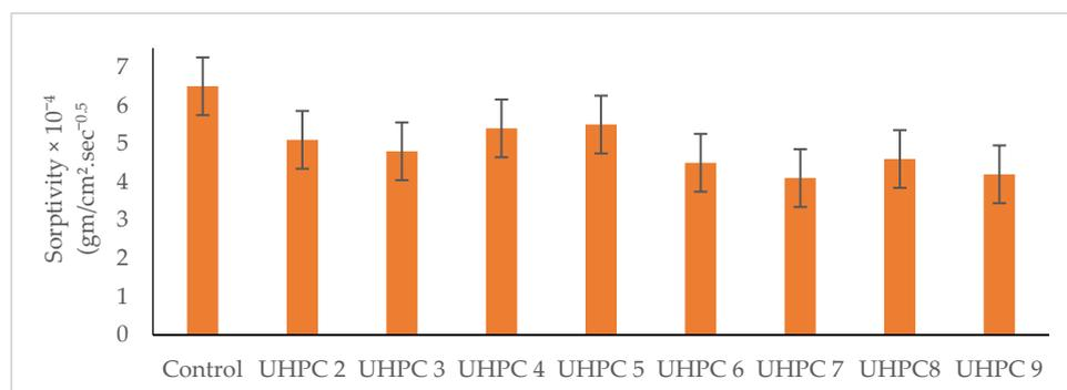
**Figure 10.** Sorptivity for glass and lime powder replacement ratios at 90 days.
