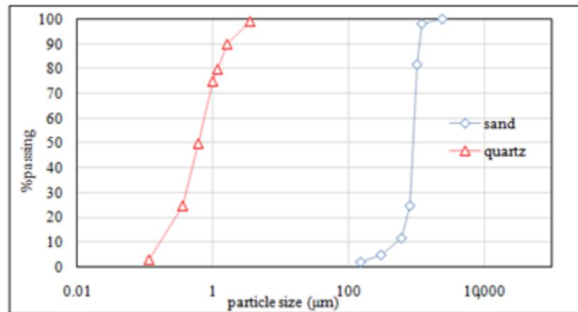
Figure 1. Quartz sand and powder distribution of particles.
