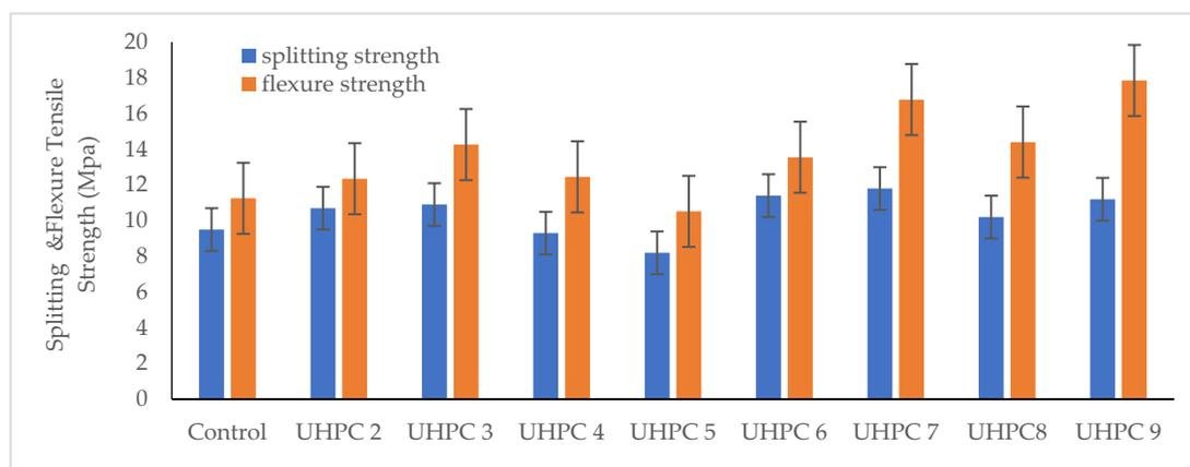
**Figure 6.** Flexural and splitting strengths after 90 days for glass and lime powder replacement ratios.
