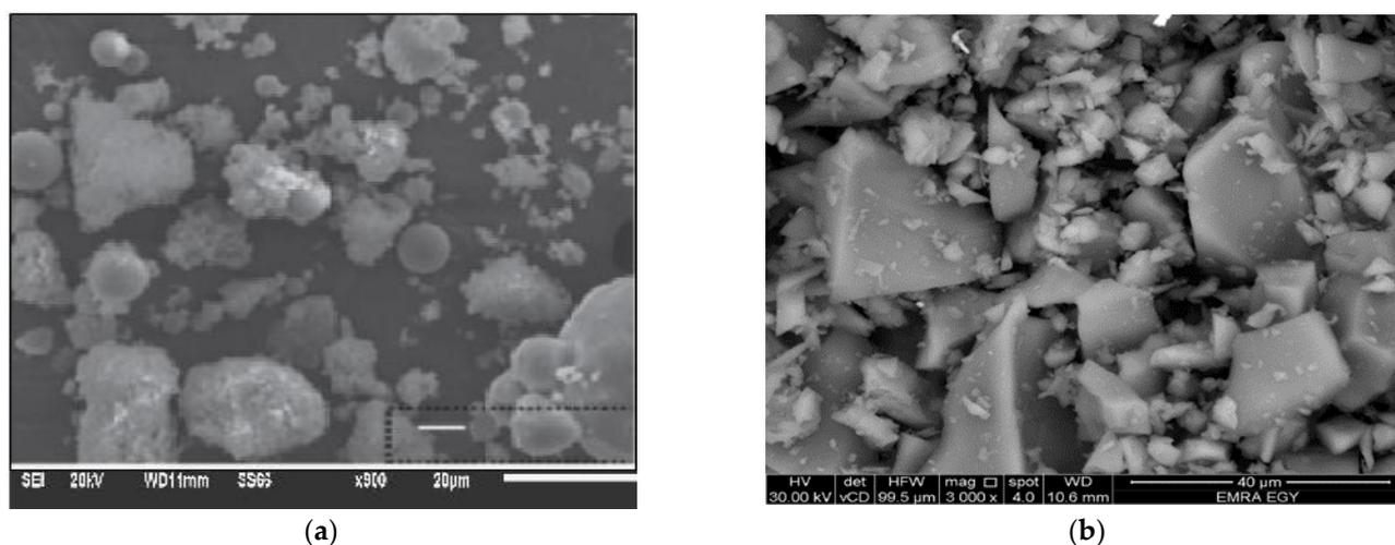
**Figure 3.** Photomicrographs of Lime and Glass powder under SEM. (a) Lime powder. (b) Glass powder.
