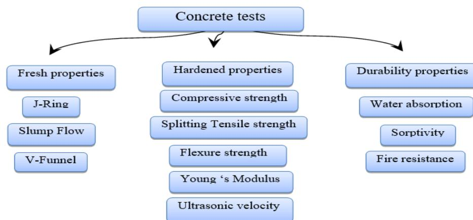
**Figure 4.** Fresh, hardened, and durability properties.
