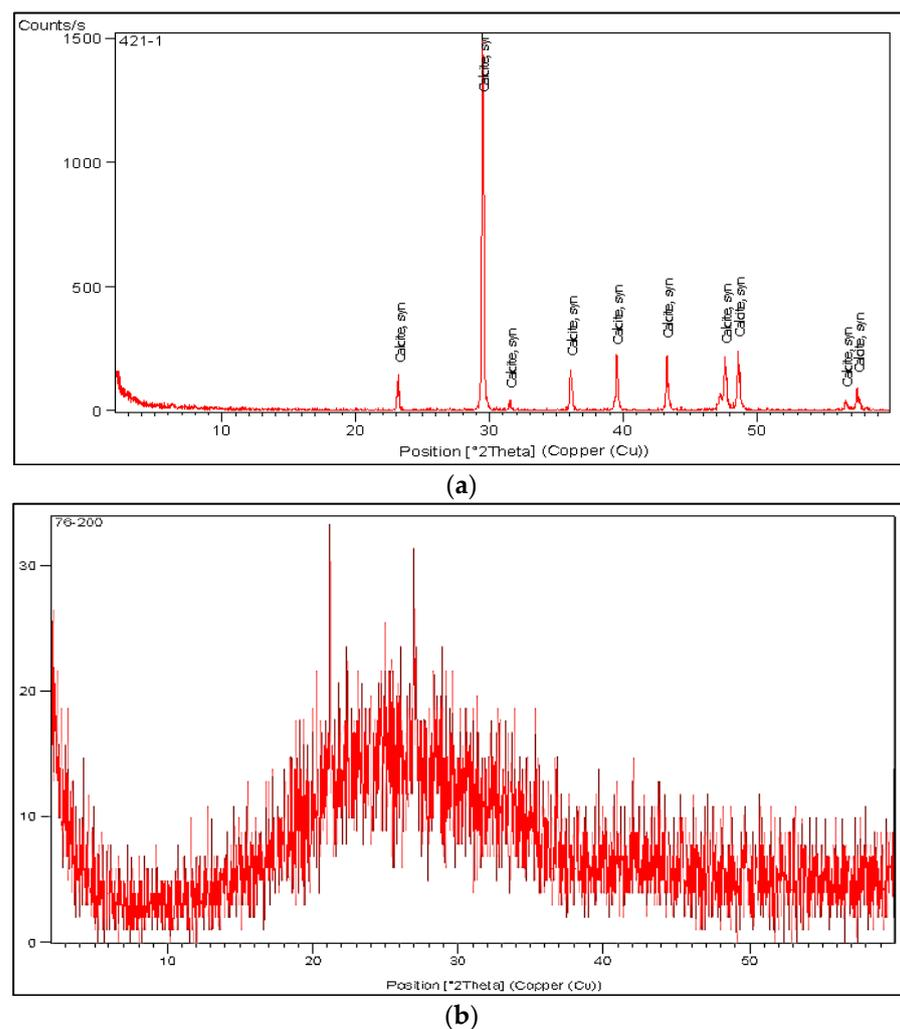
Figure 2. Lime and glass powder X-ray diffraction patterns. (a) Lime powder. (b) Glass powder.
