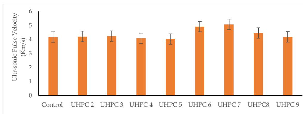
**Figure 8.** Ultrasonic pulse velocity after 90 days for glass and lime powder replacement ratios.
