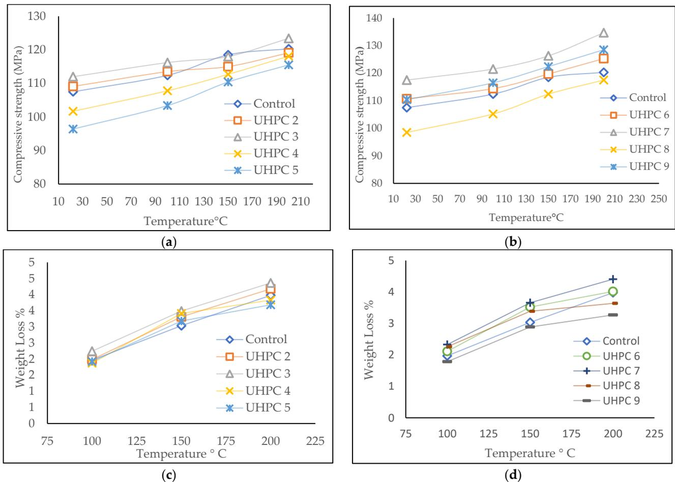
**Figure 11.** Compressive strengths and weight loss ratios under different temperatures of UHPC. (a,c) glass powder and (b,d) lime powder.
