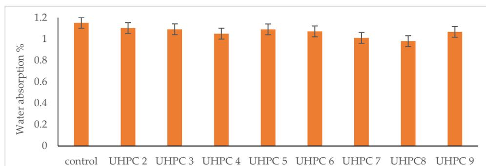
**Figure 9.** Water absorption values after 90 ages for glass powder replacement ratios.
