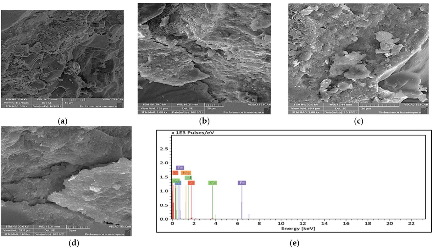
Figure 16. SEM with various magnification factors (a–d); (e) EDX for the mix UHPSCC 7 at (150 °C) temperature.
