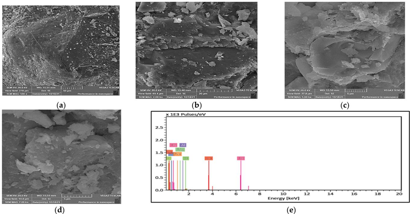
**Figure 12.** SEM with various magnification factors (a–d); (e) EDX for the control mix at 22 °C curing temperature.
