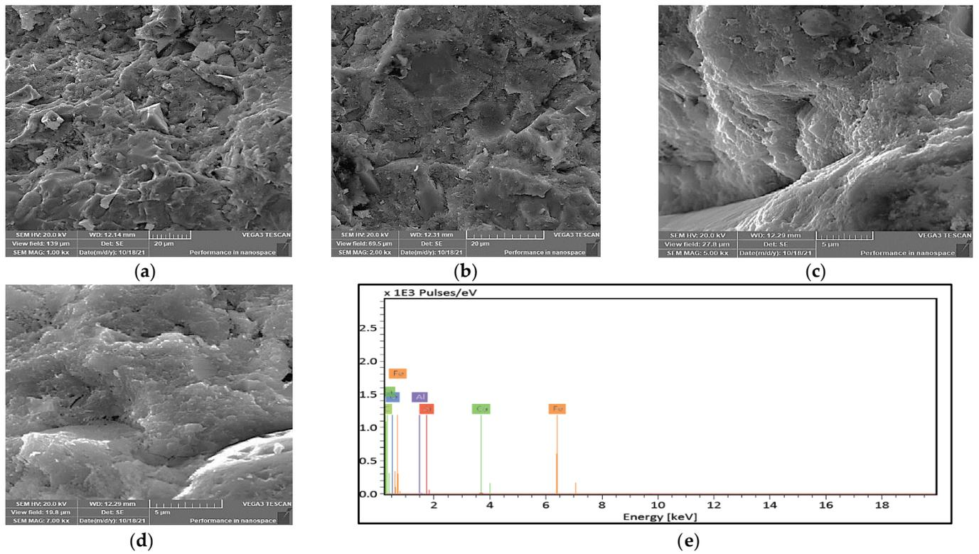
Figure 13. SEM with various magnification factors (a–d); (e) EDX for the control mix at hot curing temperature.
