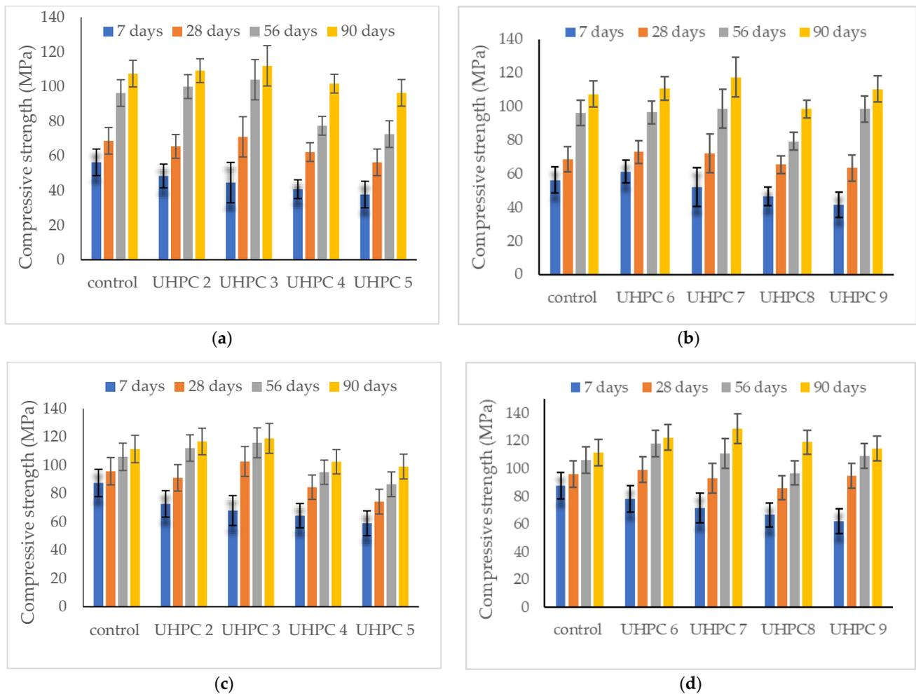
**Figure 5.** Compressive strengths of UHPC at 7,28,56, and 90 days.; (a) glass powder (N-curing), (b) lime powder (N-curing), (c) glass powder (H-curing), (d) lime powder (H-curing).
