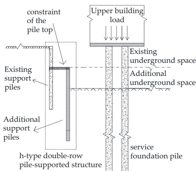
**Figure 1.** The schematic diagram of h-type double-row pile-supported structure.
