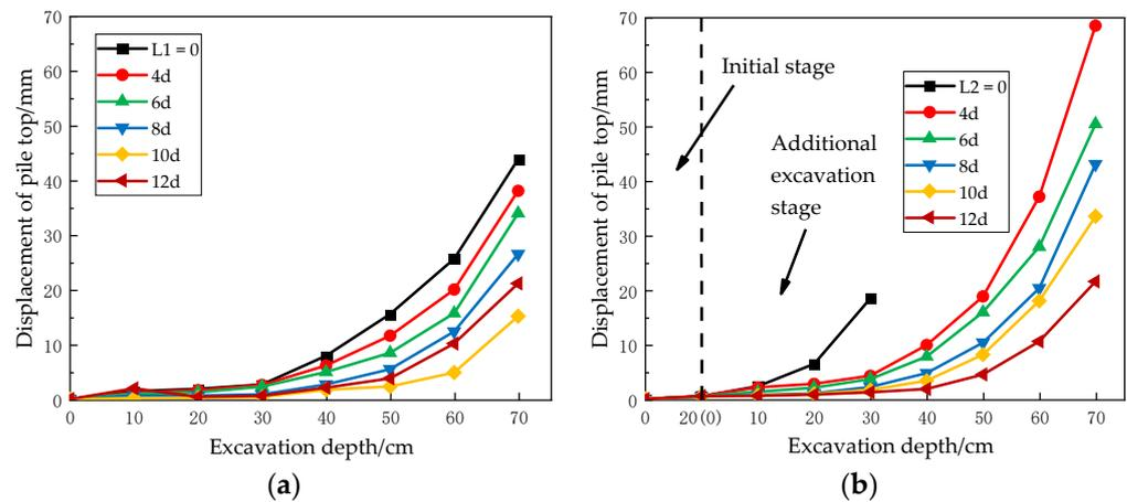
**Figure 9.** Displacement of pile top: (a) additional support piles; (b) existing support piles.
