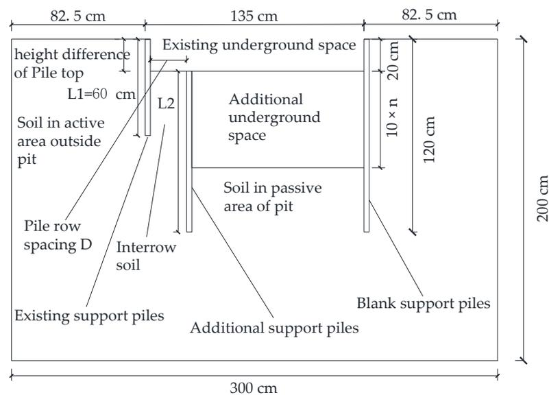
**Figure 4.** Section drawing of pile position layout.
