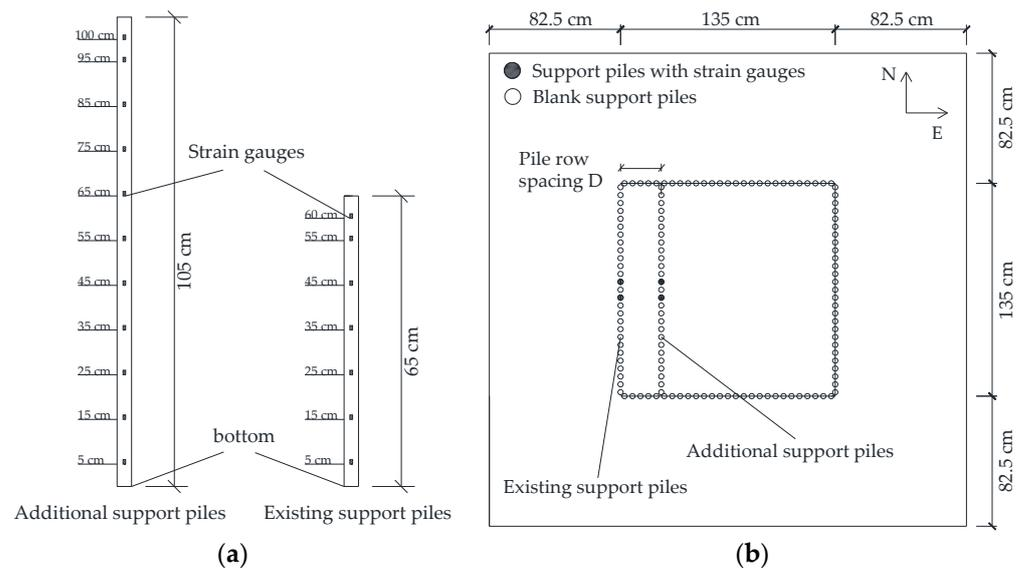
**Figure 3.** (a) Point layout diagram of strain gauges; (b) plane layout of pile positions.
