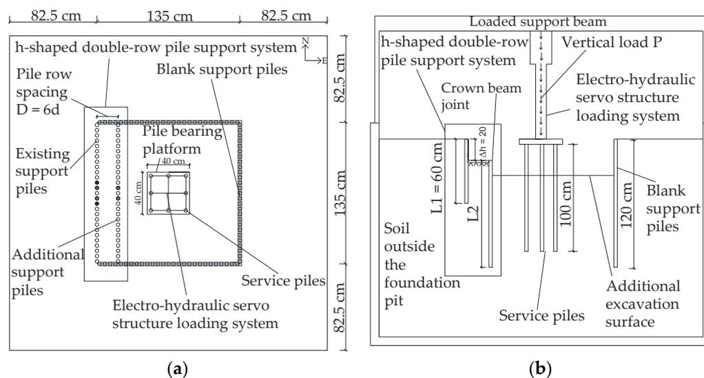
**Figure 6.** Chamber diagram for investigating the effect of service foundation piles: (a) plane graph; (b) section drawing.
