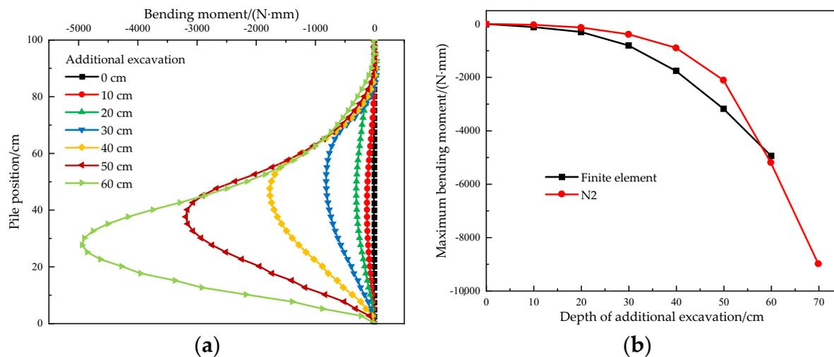
**Figure 14.** (a) Finite element bending moment diagram for additional support piles; (b) Finite element—N2 maximum bending moment comparison diagram.
