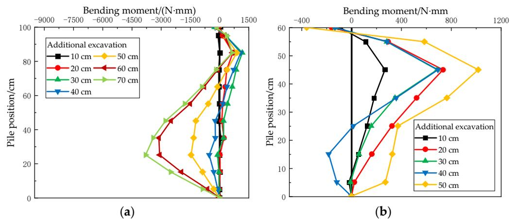
**Figure 11.** Bending moment of additional support piles: (a) group N5; (b) group N6.
