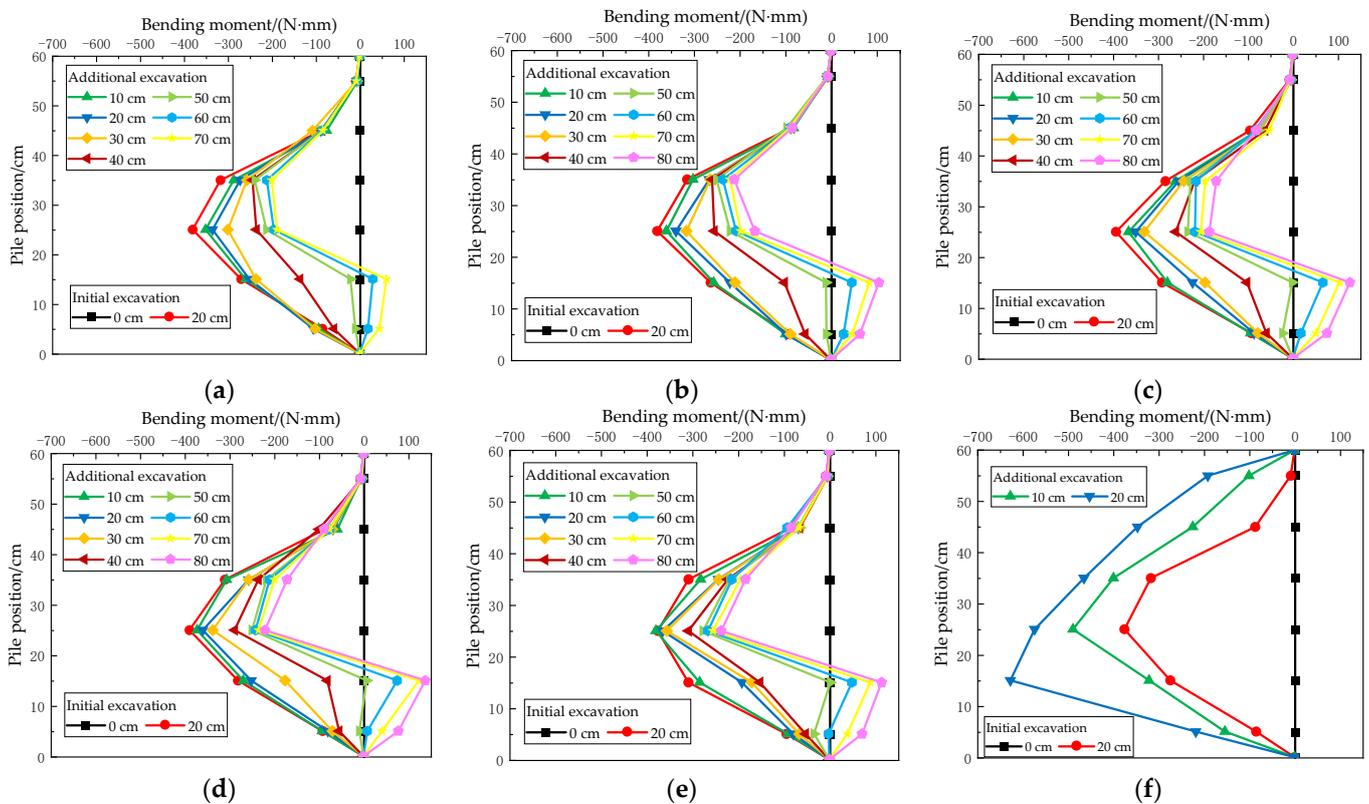
**Figure 8.** Bending moment of existing support piles: (a) group T1; (b) group T2; (c) group T3; (d) group T4; (e) group T5; (f) group T8.
