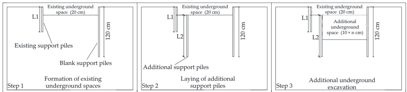
**Figure 5.** Schematic diagram of testing procedure.
