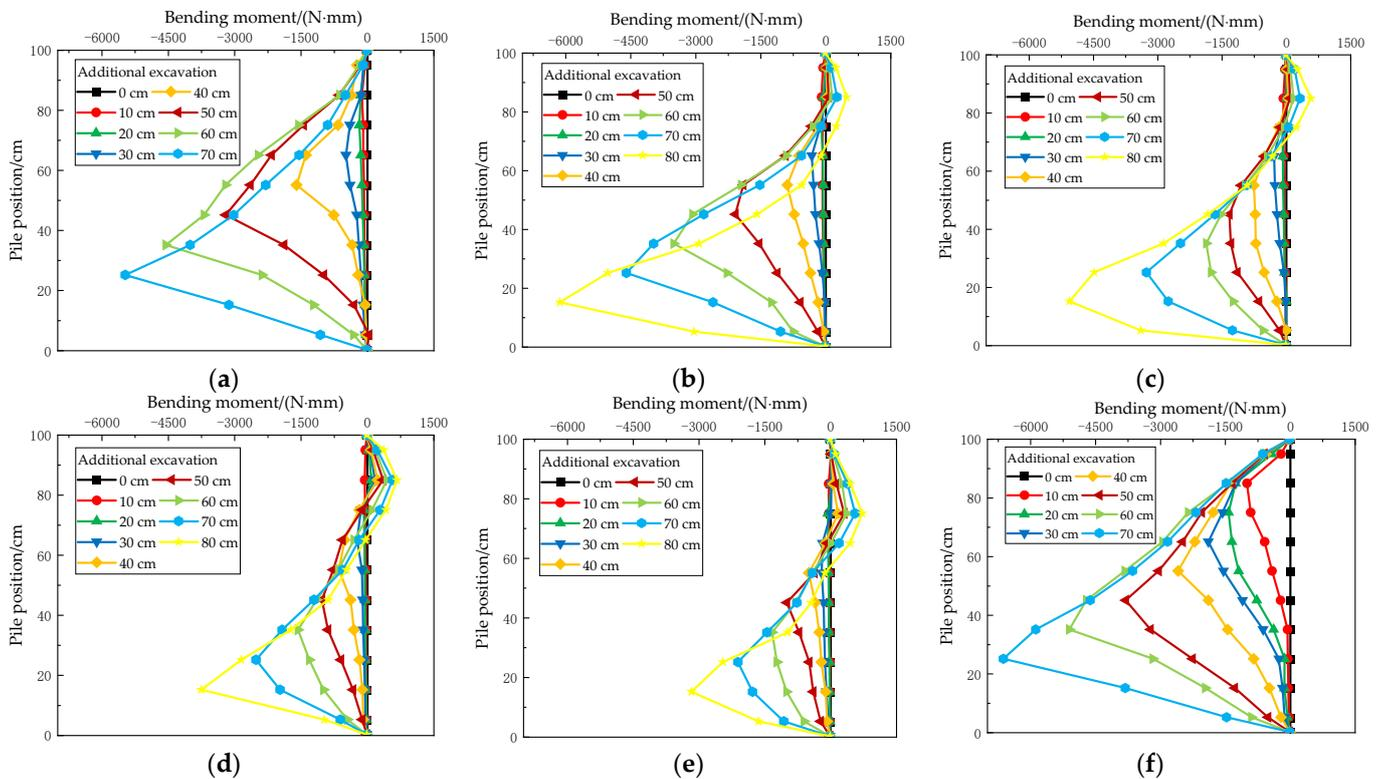
**Figure 7.** Bending moment of additional support piles: (a) group T1; (b) group T2; (c) group T3; (d) group T4; (e) group T5; (f) group T7.
