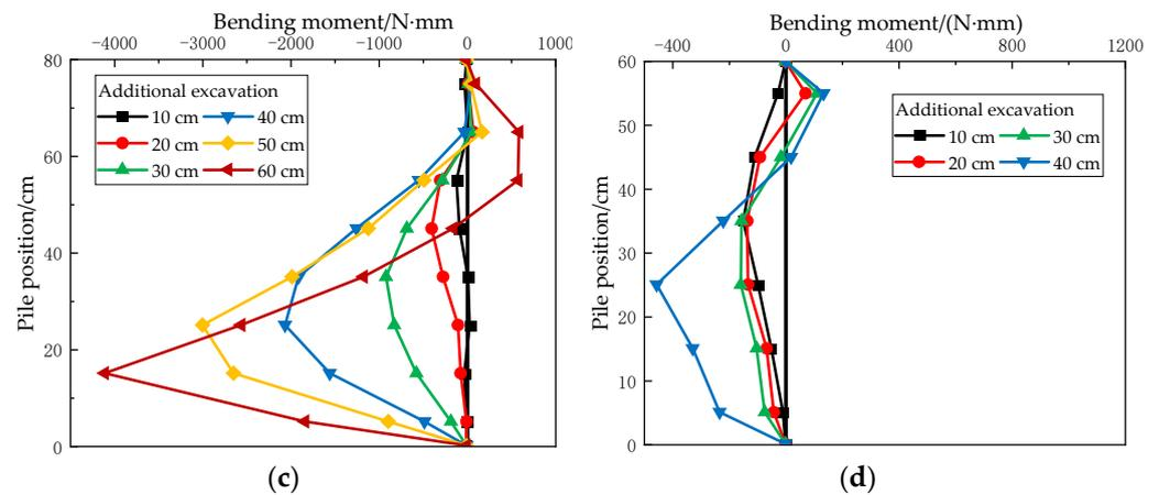
**Figure 10.** Bending moment of additional support piles under different ratios of pile length: (a) group N1; (b) group N2; (c) group N3; (d) group N4.
