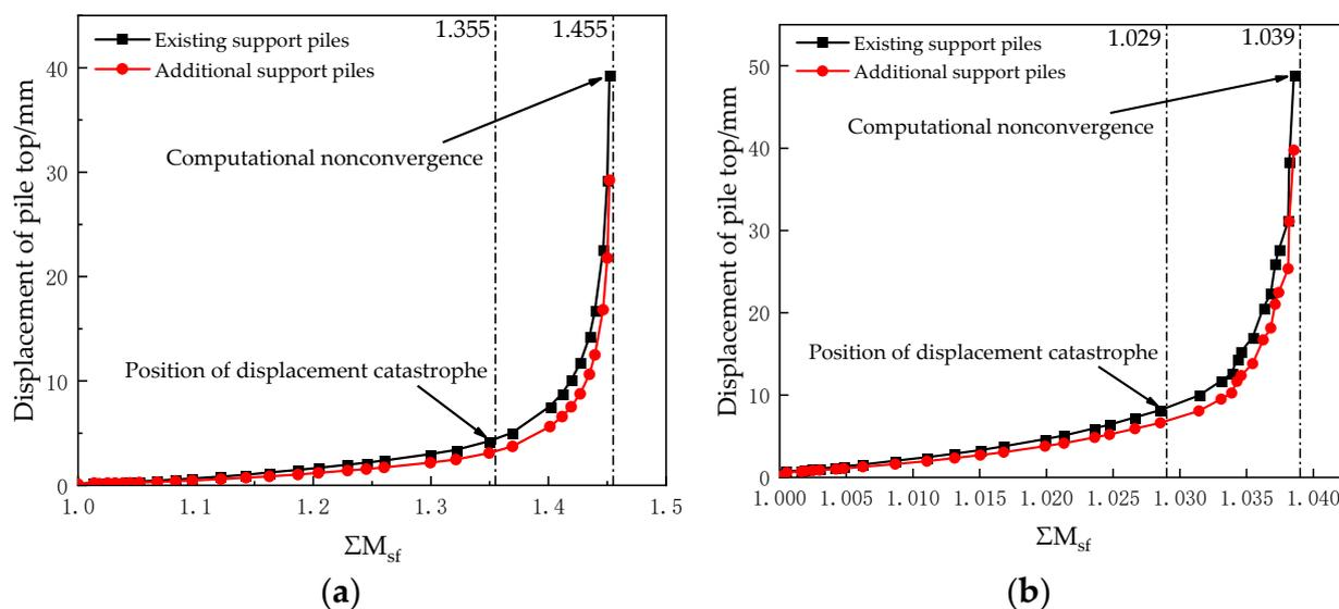
**Figure 15.** Factor of safety—displacement of pile top diagram: (a) additional excavation 40 cm; (b) additional excavation 60 cm.
