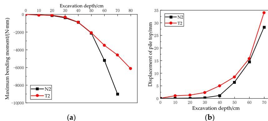
Figure 13. Comparison between maximum bending moment and displacement of pile top of N2–T2 additional support piles: (a) maximum bending moment; (b) displacement of pile top.
