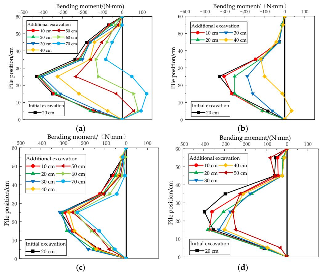
Figure 12. Bending moment of existing support piles: (a) group N2; (b) group N4; (c) group N5; (d) group N6.
