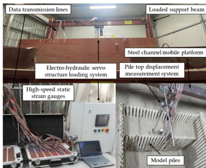
Figure 2. Main test instruments and devices.
