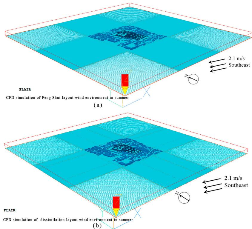
**Figure 4.** PHOENICS mesh settings: (a) the feng shui layout; (b) the dissimilation layout.
