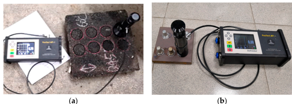
Figure 9. Pull-off test setups for (a) the with-zinc and no-zinc specimens and (b) the no-WBM and with-WBM specimens.
