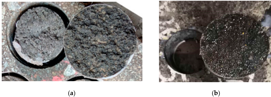
Figure 10. Interface states of specimen failure in the pull-off test: (a) the internal fracture of the concrete and (b) the interfacial fracture of the bonding layer.
