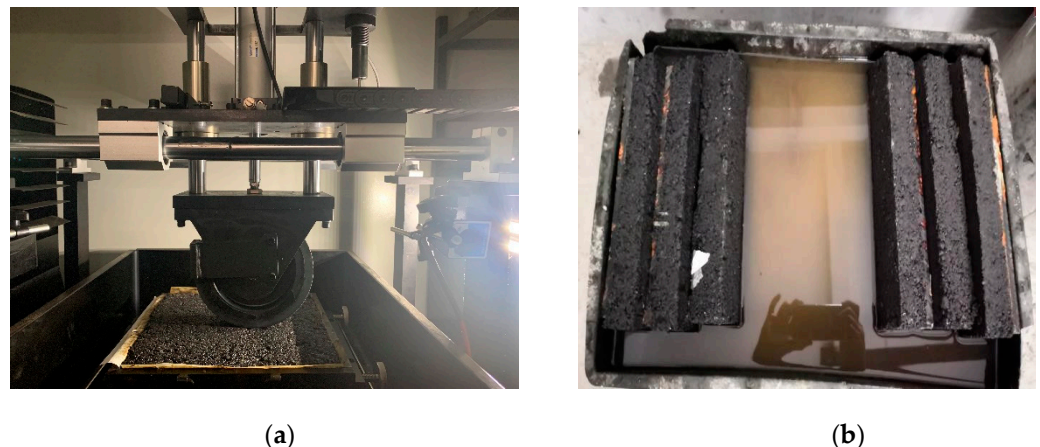
Figure 6. Setups for (a) the wheel loading test and (b) the saltwater immersion test.
