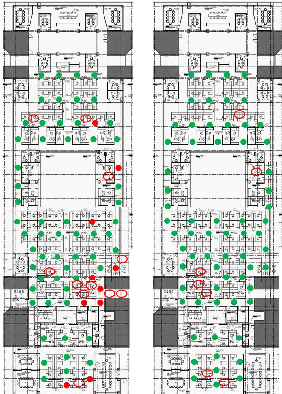
**Figure 2.** Background noise survey north wing of LEED-certified building with sound masking on (left) and off (right). The green dots denote values that met the design criteria during occupied hours whereas the red dots denote values exceeding 48 dBA. Design criteria were exceeded in some instances due to nearby conversation, denoted by the red, unfilled oval shapes.
