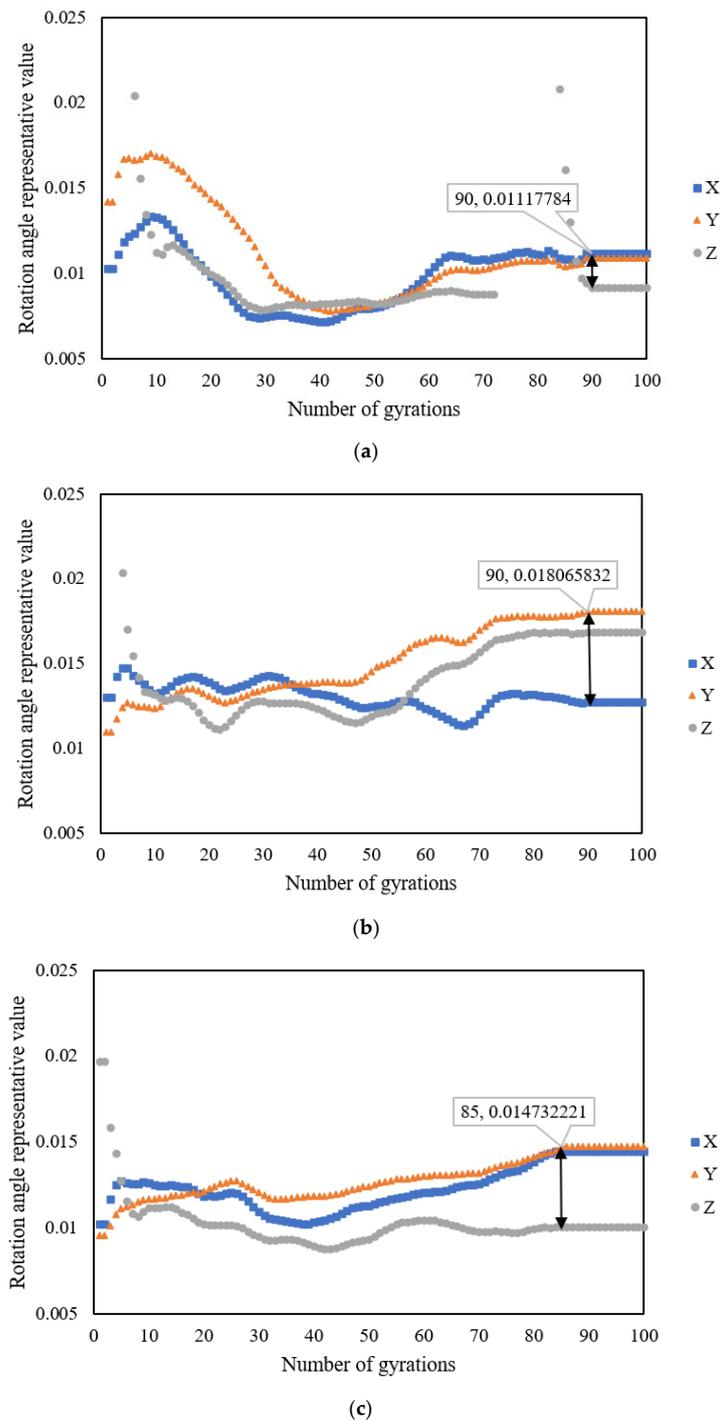
**Figure 12.** Representative rotation angle value with different compaction temperatures: (a) 160 °C, (b) 170 °C, and (c) 180 °C.
