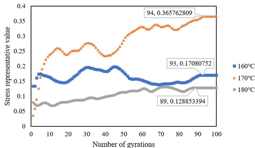
**Figure 9.** Representative stress values at different compaction temperatures.
