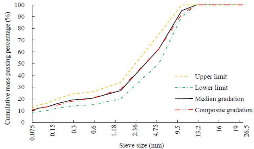
**Figure 1.** Production grading curve.
