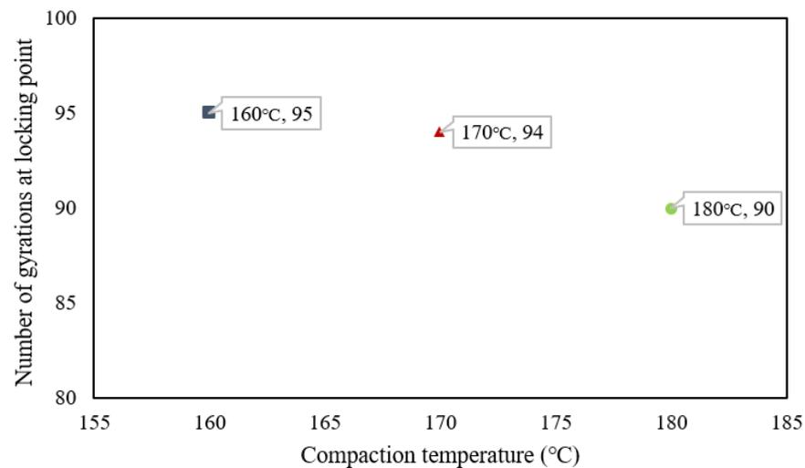
**Figure 10.** Traditional locking points with different compaction temperatures.
