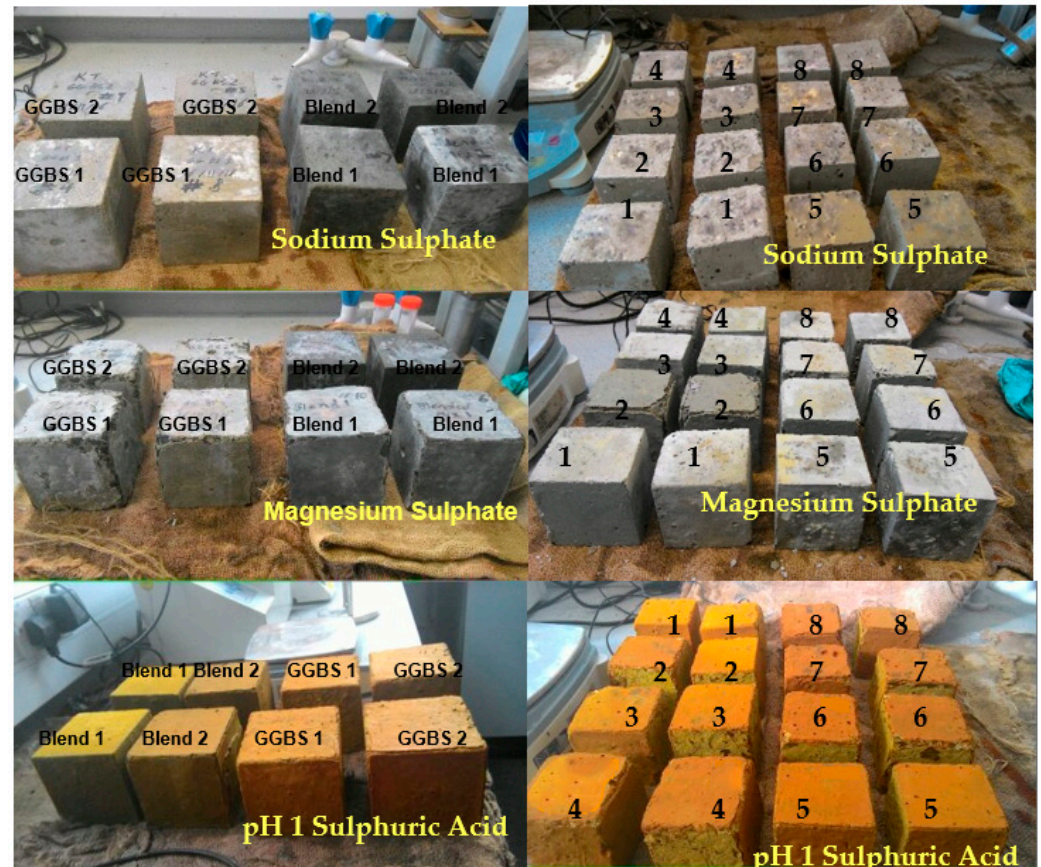
Figure 4. The visual appearance of the concrete specimens after 14 months of exposure to various solutions. Group 1 specimens are shown on the left-hand side and Group 2 on the right. The corners and edges were damaged for specimens exposed to MgSO_4 and sulphuric acid. Note the brown/orange colouration of specimens exposed to sulphuric acid.
