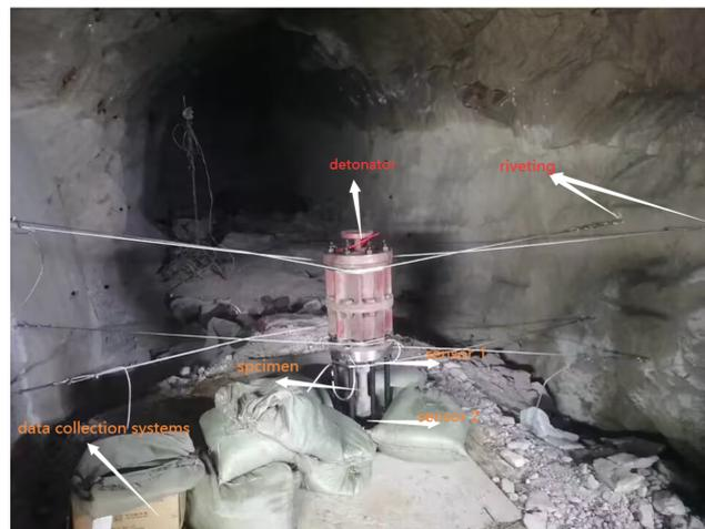
**Figure 6.** Plane explosion wave experiment sited.
