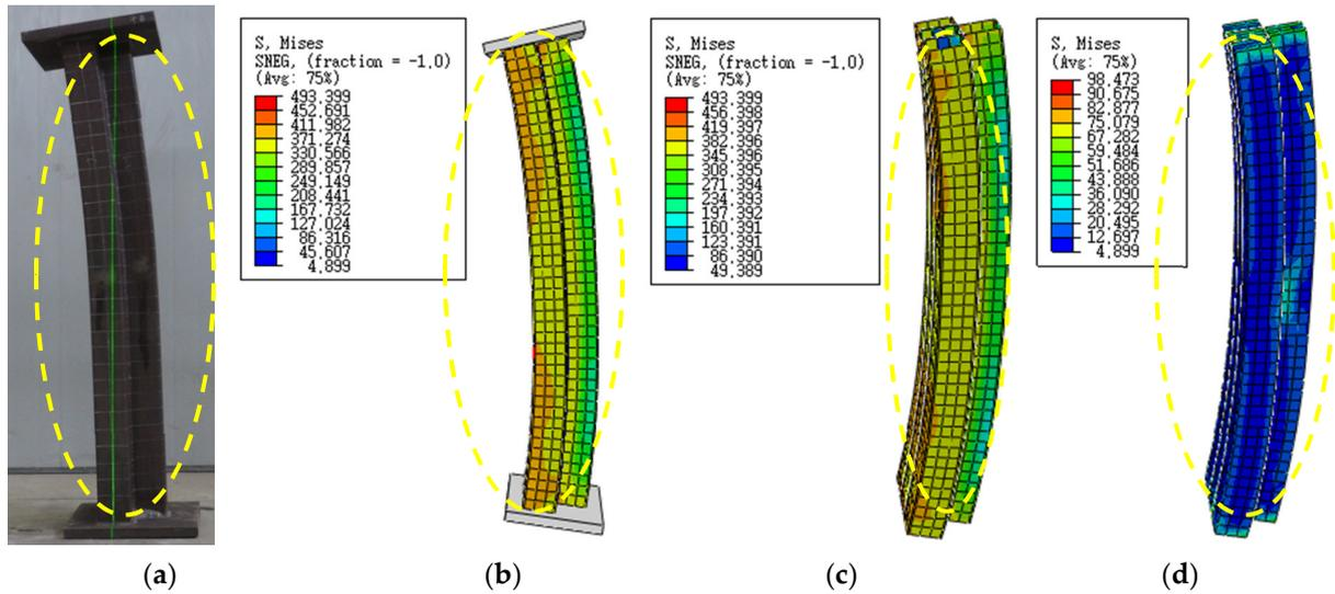
**Figure 33.** Stress distribution and failure phenomenon of finite element model of T-4 specimen: (a) Test failure mode; (b) Numerical calculation of failure mode; (c) Failure modes of steel tube; (d) Failure modes of concrete.
