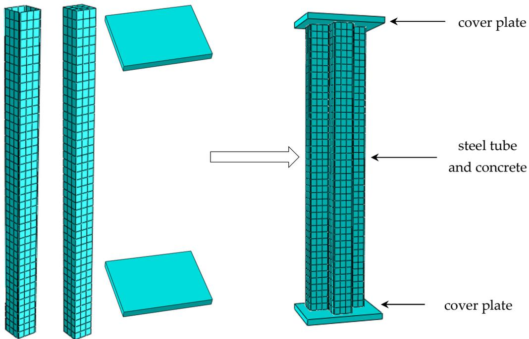
Figure 27. Elements and meshing of components.
