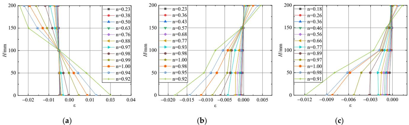
Figure 25. Strain distribution of the middle section of the pieces: (a) strain distribution in the column section of No. 2 specimen ( $e = 40$  mm); (b) strain distribution in the column section of No. 5 specimen ( $e = 40$  mm); (c) strain distribution in the column section of No. 7 specimen ( $e = 40$  mm).
