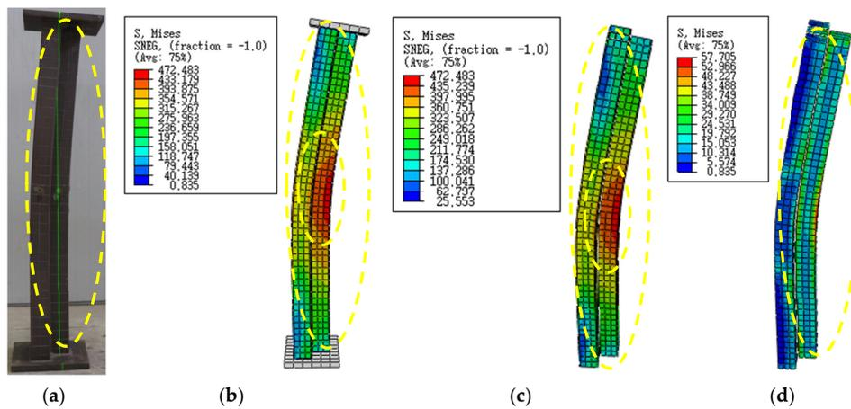
**Figure 36.** Stress distribution and failure phenomenon of finite element model of T-7 specimen: (a) Test failure mode; (b) Numerical calculation of failure mode; (c) Failure modes of steel tube; (d) Failure modes of concrete.
