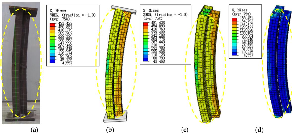
**Figure 34.** Stress distribution and failure phenomenon of finite element model of T-5 specimen: (a) Test failure mode; (b) Numerical calculation of failure mode; (c) Failure modes of steel tube; (d) Failure modes of concrete.
