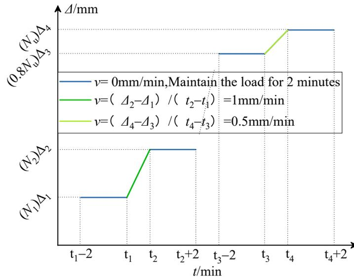
Figure 11. Test loading schematic.
