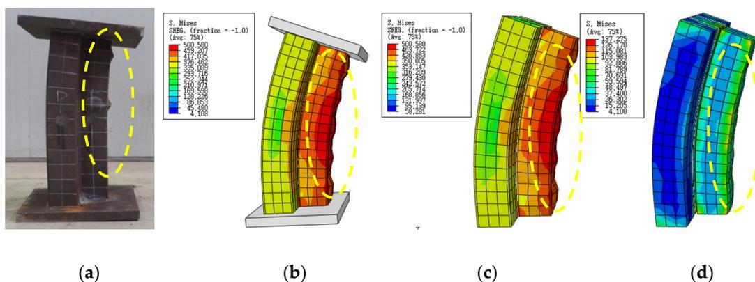
**Figure 32.** Stress distribution and failure phenomenon of finite element model of T-3 specimen: (a) Test failure mode; (b) Numerical calculation of failure mode; (c) Failure modes of steel tube; (d) Failure modes of concrete.
