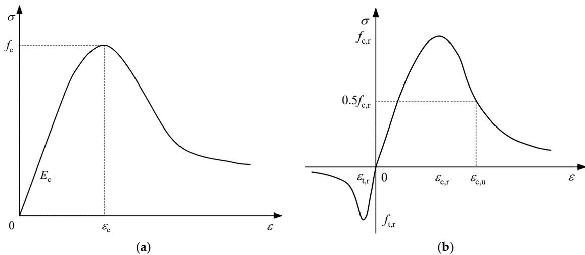
**Figure 29.** Stress–strain curve of concrete: (a) uniaxial compressive stress–strain curves for confined concrete; (b) uniaxial tensile and compressive stress–strain curves of unconstrained concrete.
