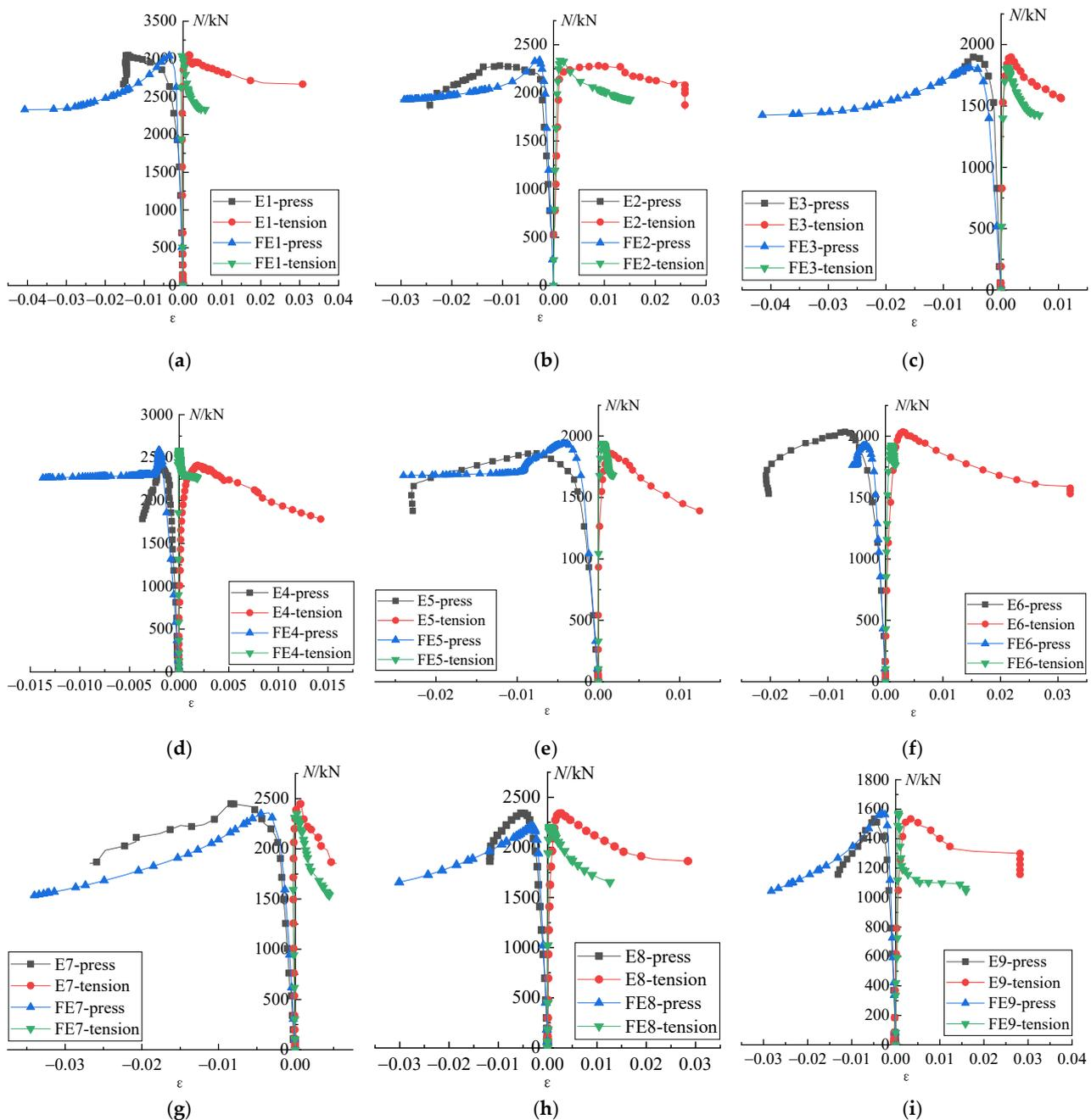
**Figure 39.** Load–strain curve of FEM: (a) load–strain curve of T-1; (b) load–strain curve of T-2; (c) load–strain curve of T-3; (d) load–strain curve of T-4; (e) load–strain curve of T-5; (f) load–strain curve of T-6; (g) load–strain curve of T-7; (h) load–strain curve of T-8; (i) load–strain curve of T-9.
