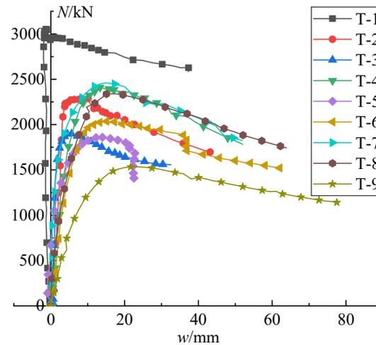
Figure 24. Load–deflection curves of specimens 1 to 9.
