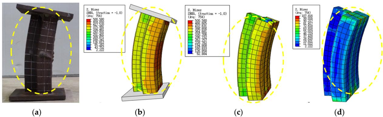
**Figure 31.** Stress distribution and failure phenomenon of finite element model of T-2 specimen: (a) Test failure mode; (b) Numerical calculation of failure mode; (c) Failure modes of steel tube; (d) Failure modes of concrete.
