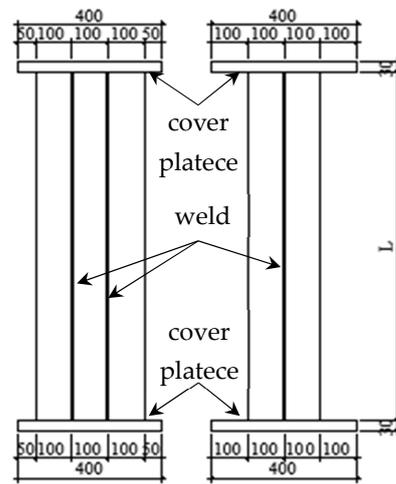
Figure 9. Design drawing of the test piece.
