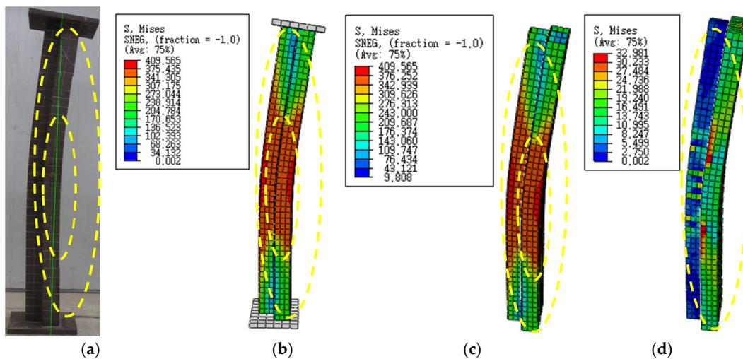
**Figure 38.** Stress distribution and failure phenomenon of finite element model of T-9 specimen: (a) Test failure mode; (b) Numerical calculation of failure mode; (c) Failure modes of steel tube; (d) Failure modes of concrete.
