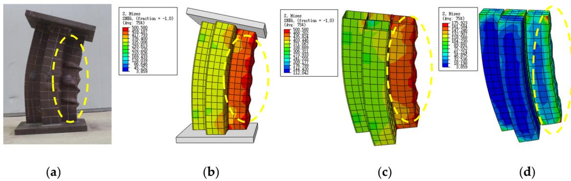
**Figure 30.** Stress distribution and failure phenomenon of finite element model of T-1 specimen: (a) Test failure mode; (b) Numerical calculation of failure mode; (c) Failure modes of steel tube; (d) Failure modes of concrete.
