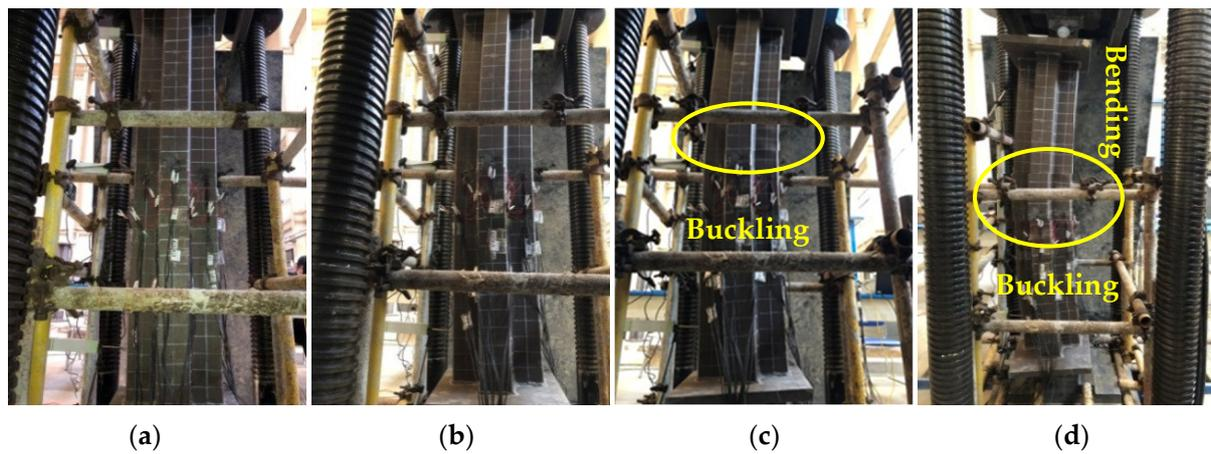
**Figure 18.** Failure process of specimen T-6: (a) Initial state; (b) Load status 1; (c) Load status 2; (d) Damage State.
