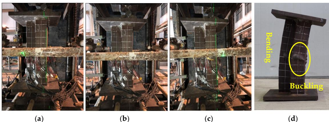
**Figure 14.** Failure process of specimen T-2: (a) Initial state; (b) Load status 1; (c) Load status 2; (d) Damage State.
