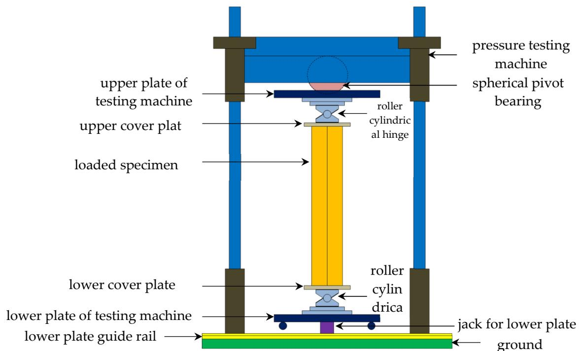
**Figure 10.** Test loading schematic.
