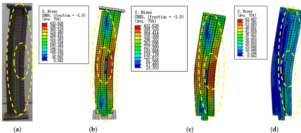
**Figure 37.** Stress distribution and failure phenomenon of finite element model of T-8 specimen: (a) Test failure mode; (b) Numerical calculation of failure mode; (c) Failure modes of steel tube; (d) Failure modes of concrete.
