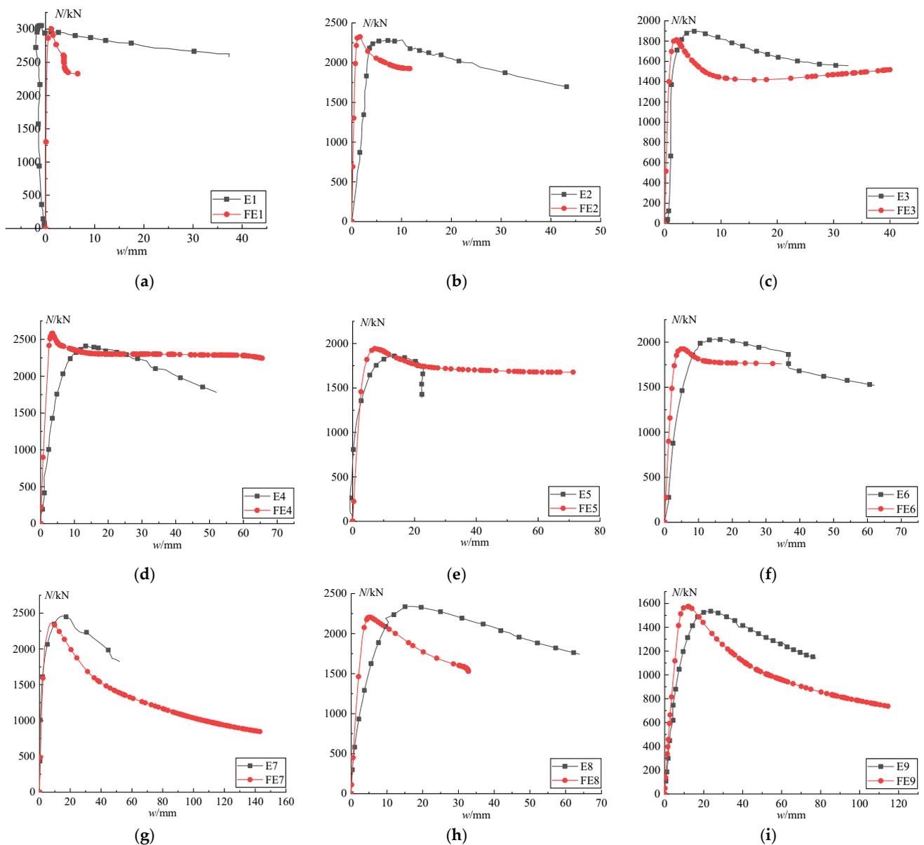
**Figure 40.** Load–deflection curve of FEM: (a) load–deflection curve of T-1; (b) load–deflection curve of T-2; (c) load–deflection curve of T-3; (d) load–deflection curve of T-4; (e) load–deflection curve of T-5; (f) load–deflection curve of T-6; (g) load–deflection curve of T-7; (h) load–deflection curve of T-8; (i) load–deflection curve of T-9.
