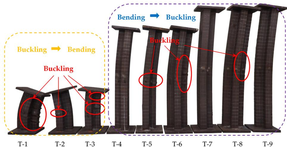
**Figure 22.** Failure results of test pieces 1 to 9.
