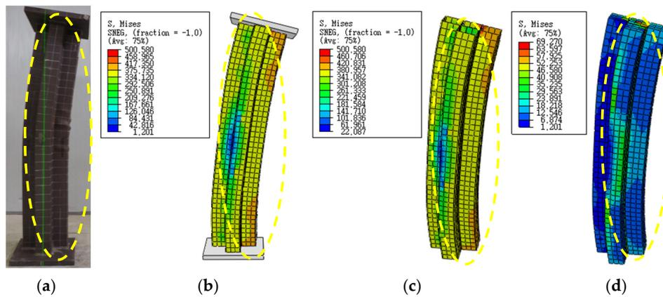
**Figure 35.** Stress distribution and failure phenomenon of finite element model of T-6 specimen: (a) Test failure mode; (b) Numerical calculation of failure mode; (c) Failure modes of steel tube; (d) Failure modes of concrete.
