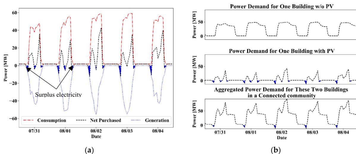
**Figure 8.** Electricity sharing in a connected community. (a) One building with PV; (b) share electricity between buildings.
