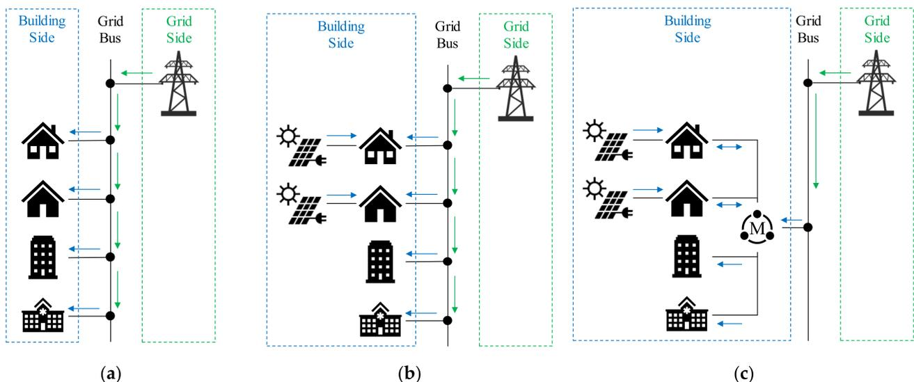
**Figure 4.** Traditional community and connected community. (a) Electricity only supplied by the grid (traditional community); (b) PV panels installed in some buildings (traditional community); (c) connected community.
