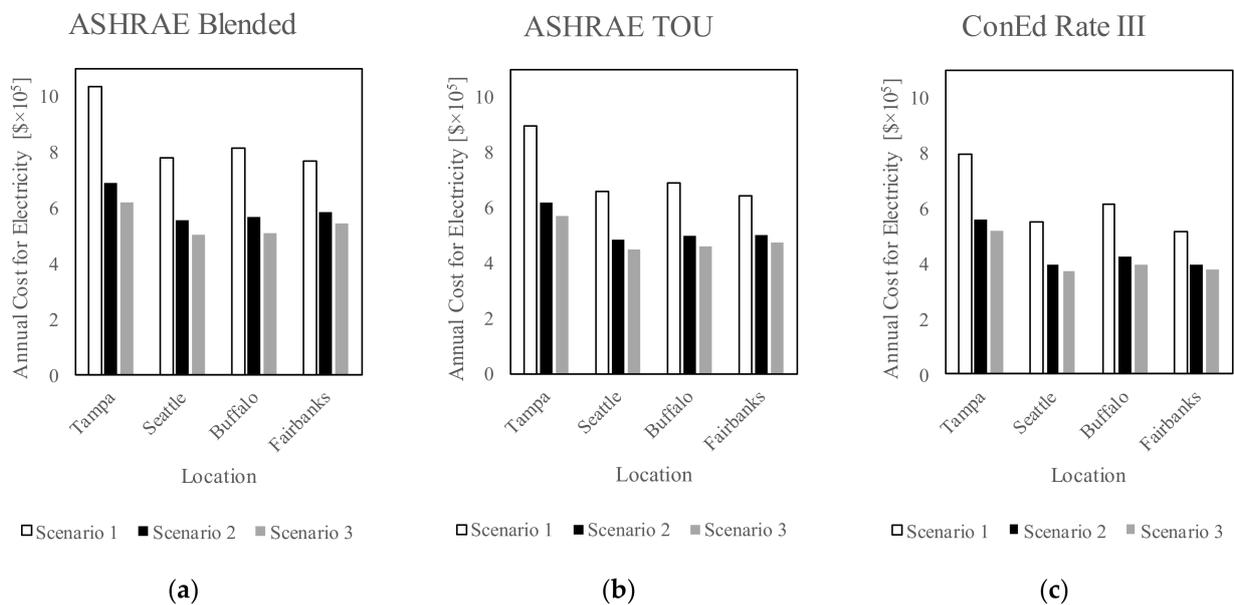
**Figure 11.** Comparison of aggregated annual electricity cost. (a) Aggregated annual electricity cost by using ASHRAE Blended electricity tariff; (b) aggregated annual electricity cost by using ASHRAE TOU electricity tariff; (c) aggregated annual electricity cost by using ConEd Rate III electricity tariff.
