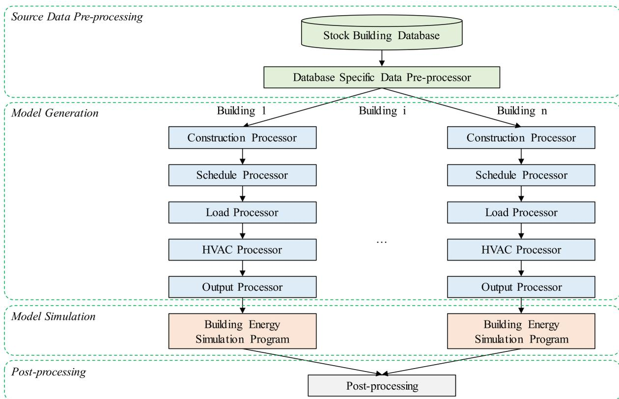
**Figure 2.** Urban-scale building energy modeling framework.
