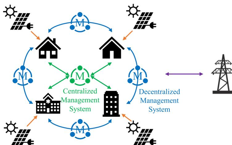
Figure 3. Implementation of the behind-the-meter DERs and management.
