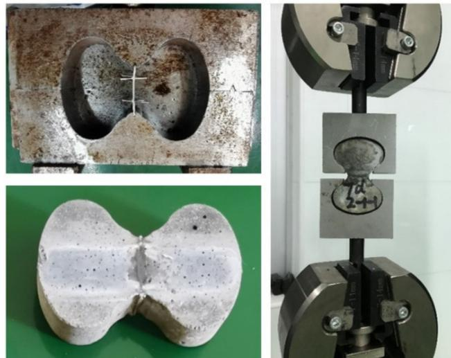
**Figure 6.** Eight-shaped mold and test method for pullout bond test.
