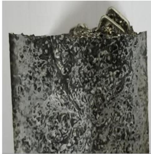
**Figure 13.** Failure mode on the fracture surface of RPC with closed steel fibers.
