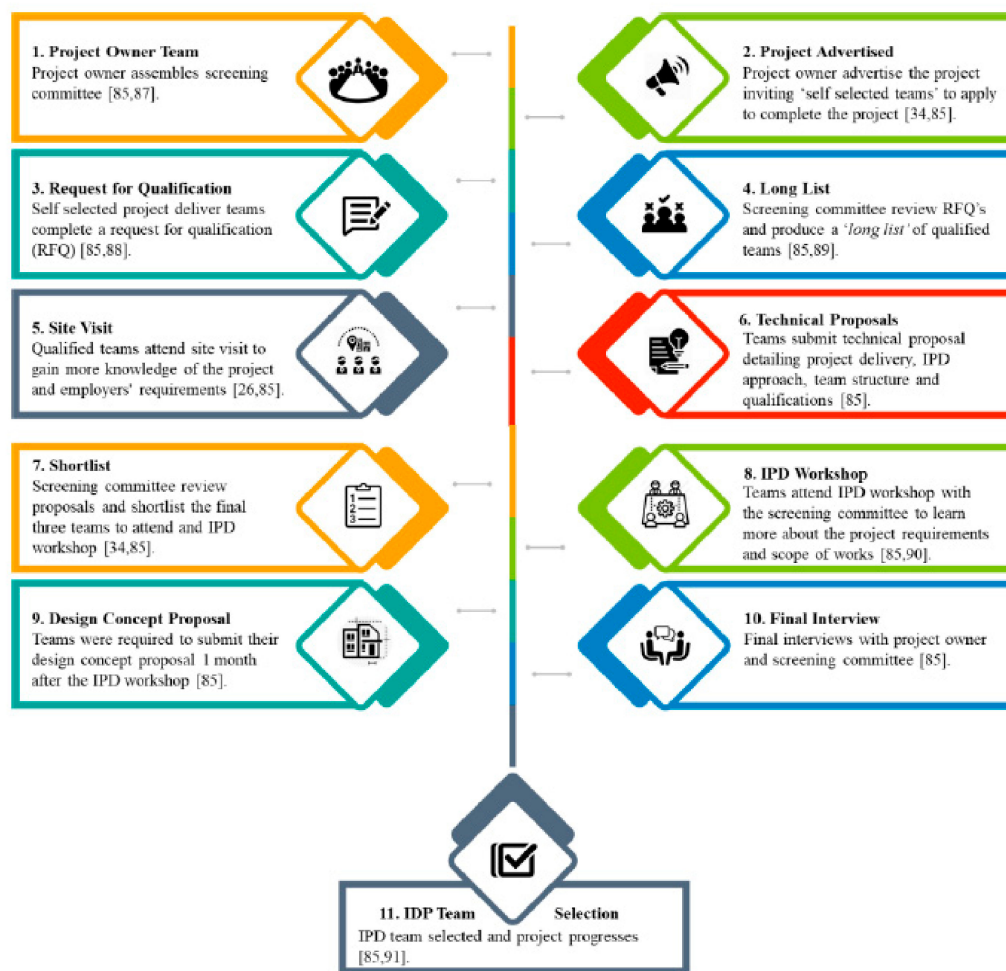
Figure 3. Integrated project delivery (IPD) selection process [26,34,85,87–91].
