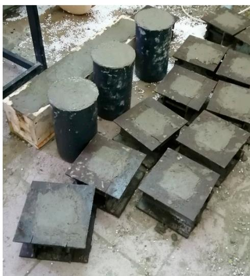
**Figure 2.** Concrete in molds.
