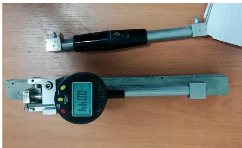
**Figure 4.** Mechanical strain gauge.
