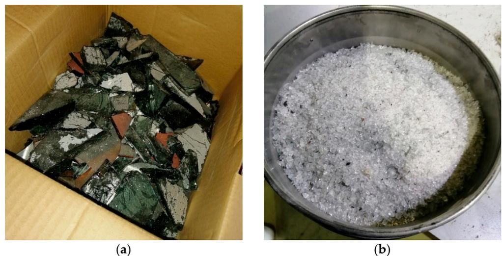
Figure 1. (a) CRT glass before crushing and (b) after crushing.
