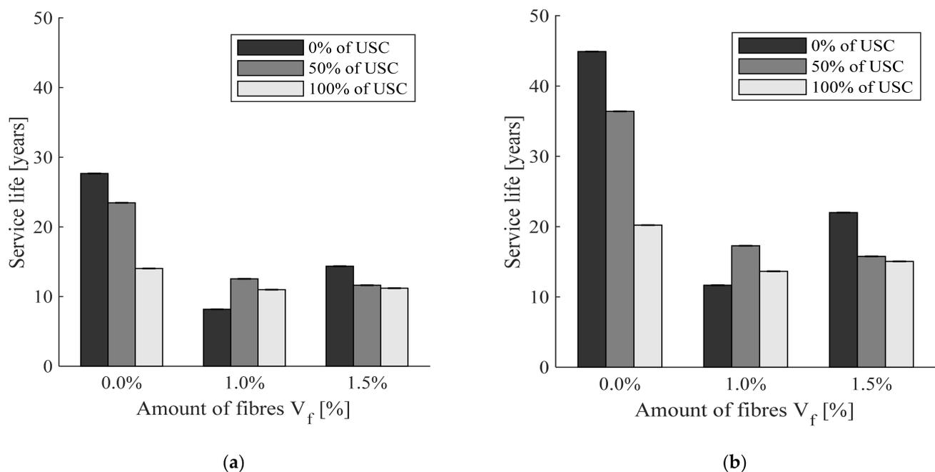
**Figure 6.** The service life regarding (a) the constant diffusion coefficient and (b) the time-dependent diffusion coefficient.
