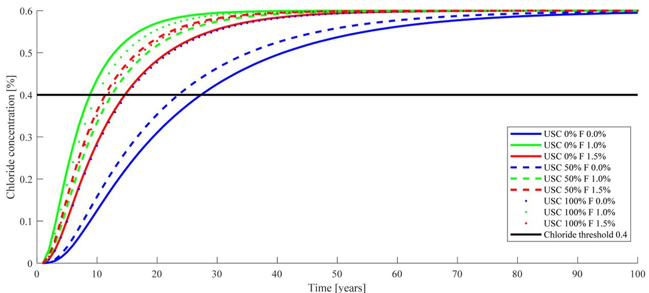
**Figure 4.** Chloride concentration over time regarding the constant diffusion coefficient.
