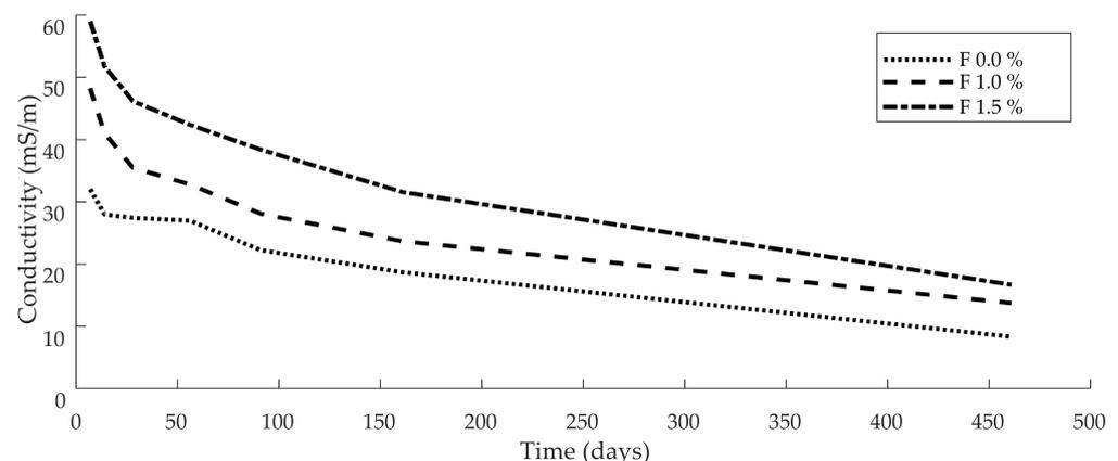
**Figure 1.** Conductivity of the SLWAC in time with different amounts of fibres.
