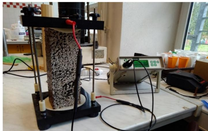
**Figure 2.** Testing of the bulk resistivity with RCON [14].
