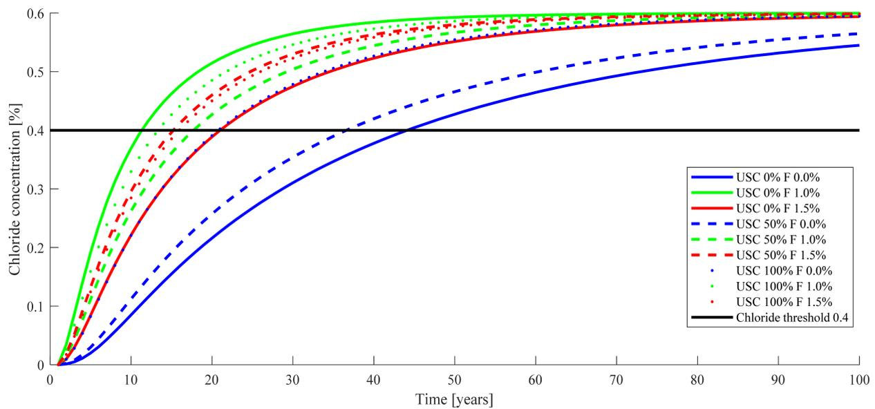
Figure 5. Chloride concentration over time regarding the time-dependent diffusion parameters.
