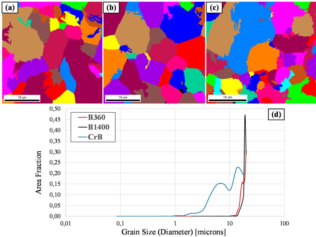
**Figure S2.** (a) Grain map showing the PAGs for B360-HT, (b) PAGs for B1400-HT, (c) PAGs for CrB-HT, (d) the grain size distribution for all steels.
