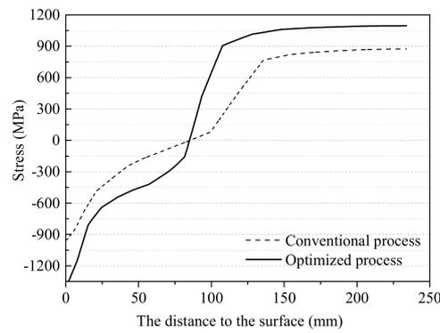
Figure 4. The residual axial stress distribution curves.
