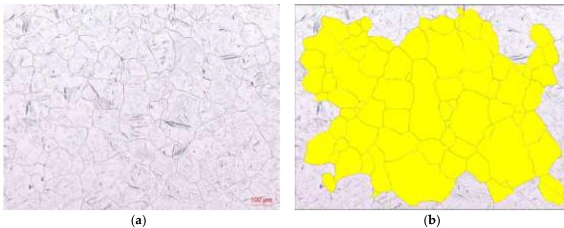
**Figure 1.** (a) Initial image of austenite obtained using optical microscopy and (b) after the detection process using analysis software after quenching.
