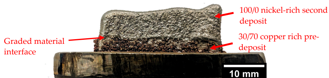
Figure 9. Copper–nickel FGM deposit fabricated with 30/70 as the pre-deposit and 100/0 as the second deposit. The set 3 duty cycle rampdown parameter was used at the dissimilar material interface.
