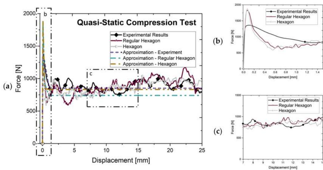
**Figure 10.** (a) The results from the implicit simulations with the regular hexagonal and hexagonal cells referenced to force results from the quasi-static experiment; (b) close-up of the peak of force; and (c) close-up of the results in the plateau range.
