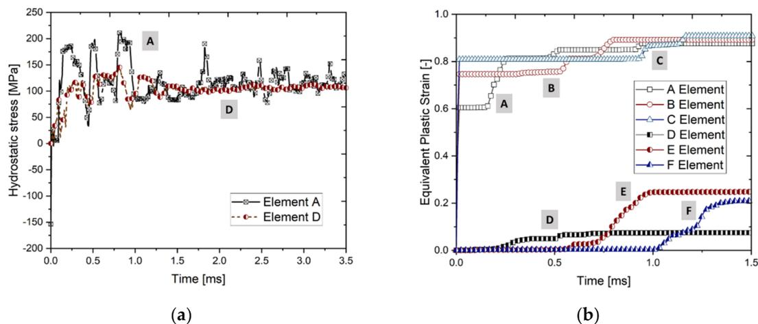
**Figure 17.** (a) Hydrostatic stresses in time for the element chosen on the double (A) and the single wall (D) from the folds formed as the first, and (b) evolution of the equivalent plastic strain for the six chosen elements.
