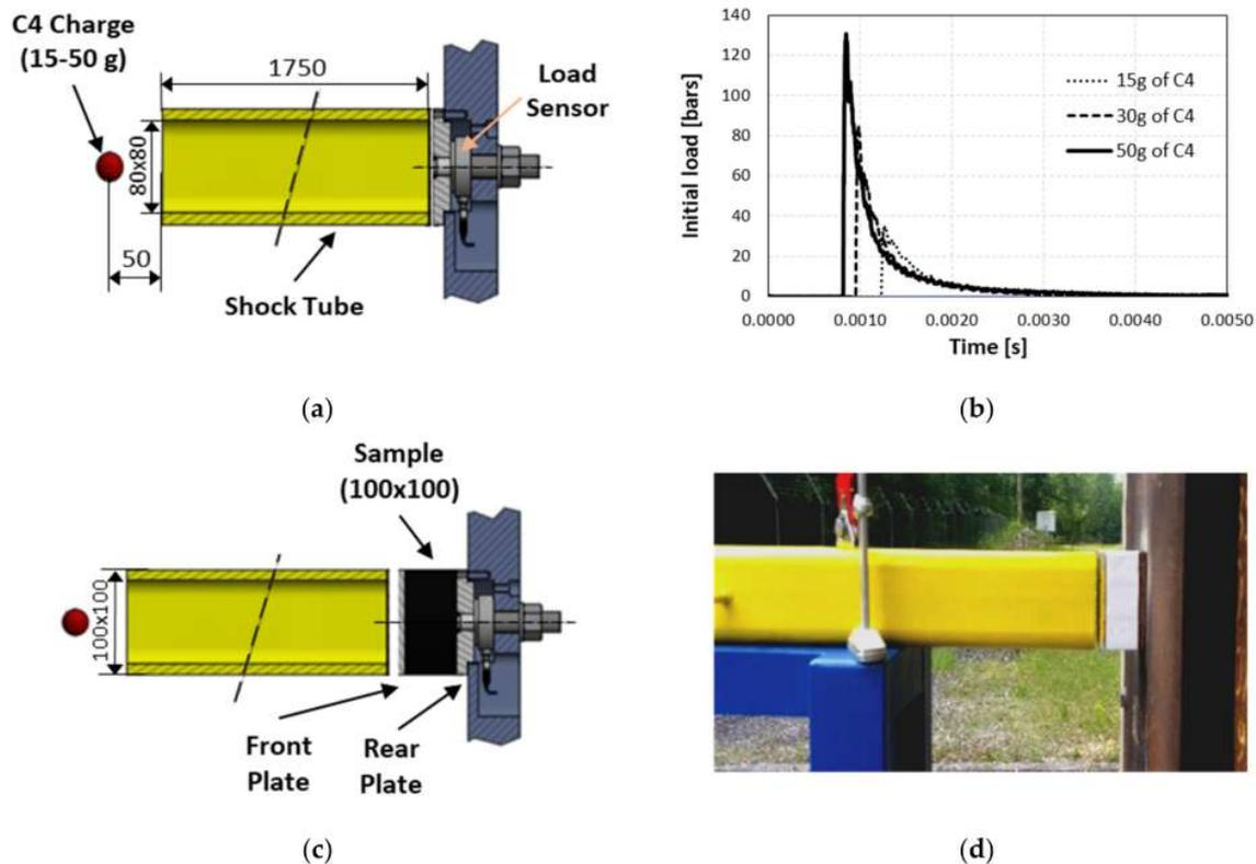
**Figure 3.** Explosive-driven shock tube: (a) scheme of the experimental configuration used to measure a blast wave pressure without application of an energy-absorbing structure, (b) measured blast wave pressures  $p(t)$  generated by detonation of several C4 charges, (c) scheme of a test with an energy-absorptive structure and (d) picture of the set-up. Dimensions are in mm.
