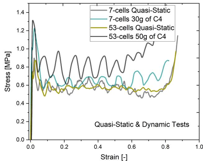
**Figure 7.** Comparison of the stress-strain curves resulted from quasi-static and blast-induced compression.
