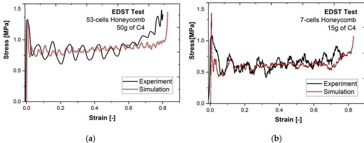
**Figure 12.** Comparison between stress–strain curves obtained in the simulation and in the EDST blast test for (a) a 53-cell structure compressed in detonation of 50 g C4 and (b) 7-cell structure compressed in the detonation of 15 g C4.
