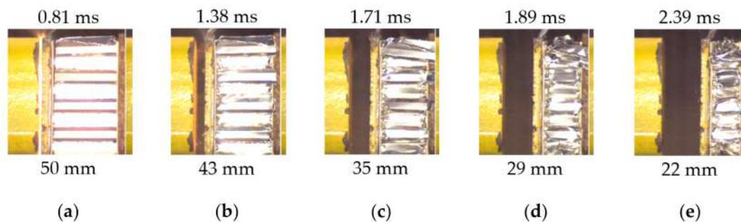
**Figure 4.** Subsequent frames depicting compression of the honeycomb during the explosive-driven shock tube (EDST) blast test: (a–e) Different decrease of the sample height (bottom row) and different recording time (upper row).
