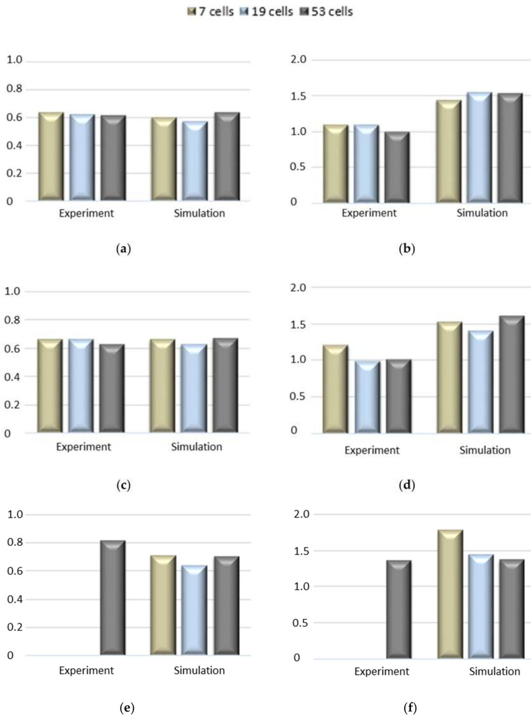
**Figure 13.** Comparison between the experimental and numerical mean and peak stresses characteristic for the structural responses to compression caused by the detonation of various masses of C4: (a) 15 g of C4, mean stress; (b) 15 g of C4, peak stress; (c) 30 g of C4, mean stress; (d) 30 g of C4, peak stress; (e) 50 g of C4, mean stress; (f) 50 g of C4, peak stress.
