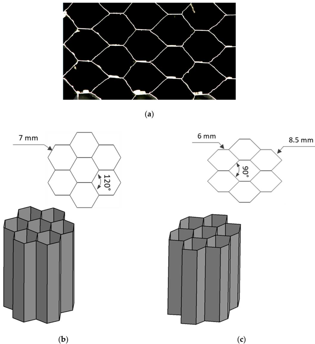
**Figure 9.** Comparison of cells of the honeycomb structure: (a) top-view on the real sample, (b) geometry idealized by “regular hexagon” cells, and (c) “hexagonal” cells with dimensions closer to the real ones.
