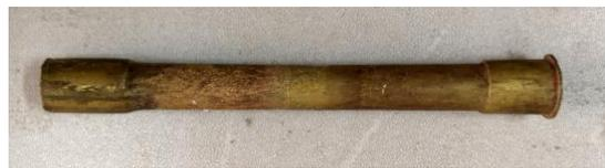
Figure 3. Copper tube after explosive consolidation.
