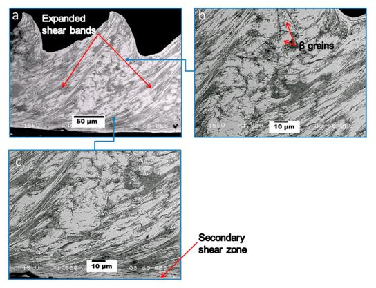
**Figure 2.** SEM of machining chip microstructure for surface cutting speed around 90 m/min: (**a**) Low magnification image of segmented chip morphology. (**b**) Undeformed chip region with original  $\beta$  grain structure of the workpiece material with in-tact  $\beta$  grains highlighted. (**c**) Higher magnification image of the secondary shear zone which adjoins the tool rake face during cutting.
