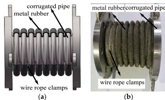
**Figure 1.** (a) Schematic diagram of the coated damping structure for metal rubber of bellows; and (b) physical picture of coated damping structure for metal rubber of bellows.
