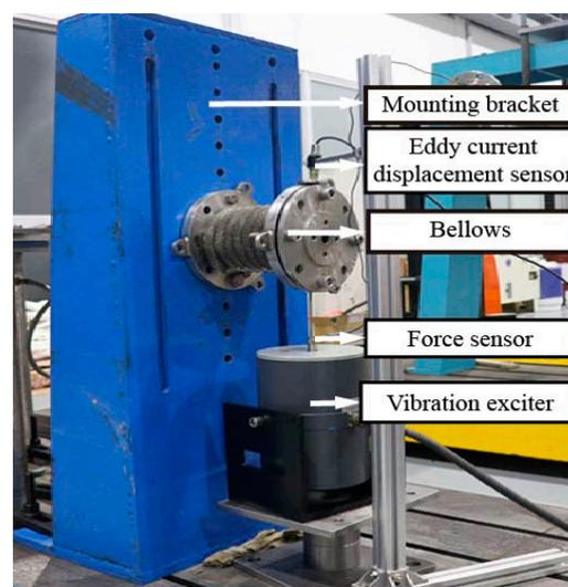
Figure 3. The test device.
