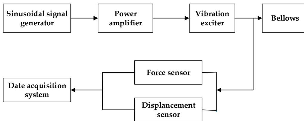
**Figure 4.** Principle of dynamic test for coated damping structure for metal rubber of bellows.
