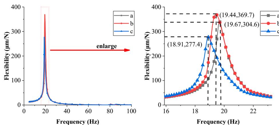
**Figure 5.** Frequency sweeping test results. Line a: Frequency sweeping curve for  $\approx 5$ –100 Hz (exciting force = 1 N); Line b: Frequency sweeping curve for  $\approx 100$ –5 Hz (exciting force = 1 N); Line c: Frequency sweeping curve for  $\approx 5$ –100 Hz (exciting force = 3 N).
