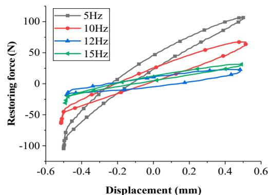
Figure 6. Hysteresis loop at different frequencies  $f$  ( $A = 0.5$  mm).
