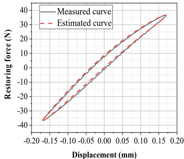
**Figure 12.** Comparison between the measured curve and estimated curve (vibration amplitude = 0.172 mm, frequency = 5 Hz).
