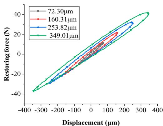
Figure 7. Hysteresis loop at different amplitudes  $A$  ( $f = 10$  Hz).
