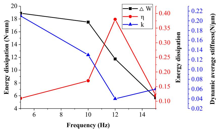
Figure 8. Test data processing results of group 1 (A = 0.5 mm).
