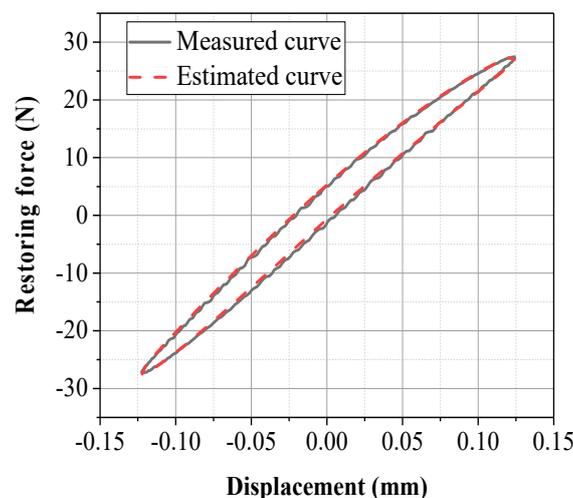
**Figure 11.** Comparison between the measured curve and estimated curve (vibration amplitude = 0.125 mm, frequency = 5 Hz).
