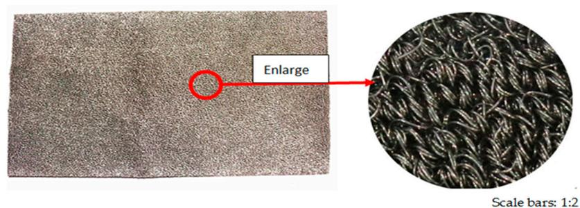
Figure 2. Large-size metal rubber sheets.
