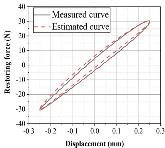
**Figure 13.** Comparison between the measured curve and estimated curve (vibration amplitude = 0.350 mm, frequency = 10 Hz).
